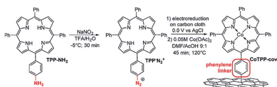
Scheme 2 Preparation of covalently immobilized Co tetraphenylporphyrin (CoTPP-cov). 121 Copyright (2019) Elsevier.
