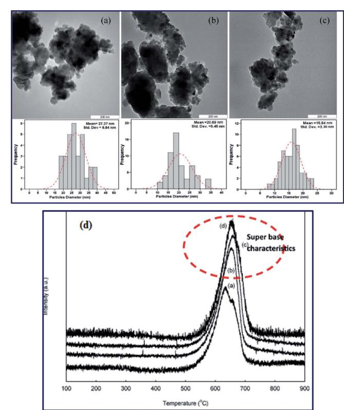
Fig. 17 TEM images and particle size distributions of the surfactant assistant CaO nanocatalysts: after 40 min (a), after 80 min (b), and after 120 min (c).  $CO_2$  desorption performance commercial of CaO (a), and nano CaO catalysts: after 40 min (b), after 80 min (c), and after 120 min (d). Reproduced from ref. 202.
