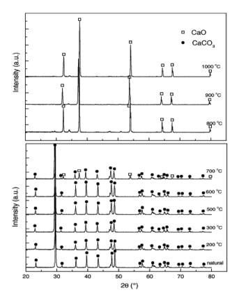
Fig. 12 XRD patterns of natural eggshell and the materials obtained by calcining natural eggshell in the range of 200–1000 °C. Reproduced from ref. 161.
