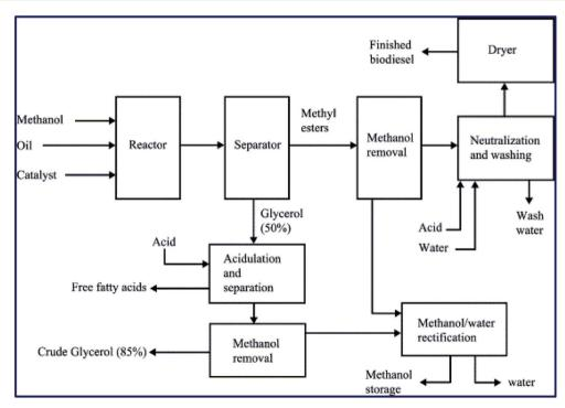
Fig. 36 Representative diagram for biodiesel production. Reproduced from ref. 447.
