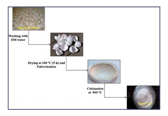
Fig. 16 Schematic layout for eggshell-originated CaO synthesis. Reproduced from ref. 192.
