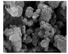
Fig. 5 SEM micrographs of (a) Hβ and (b) 30% SiW<sub>12</sub>/Hβ. Reproduced from ref. 101.
