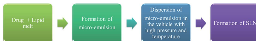
Chart 2 Preparation of solid lipid nanoparticles by oil/water (o/w) microemulsion method.
