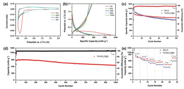
Fig. 5 CV curves (a) of YS-SiO<sub>x</sub>/C@C in the potential range of 0.01–2.0 V vs. Li<sup>+</sup>/Li at 0.1 mV s<sup>-1</sup>, selected galvanostatic charge–discharge profiles (b) of YS-SiO $_x$ /C@C at 100 mA g $^{-1}$ , cycling performances (c) of YS-SiO $_x$ /C@C and SiO $_x$ /C at 100 mA g $^{-1}$ , long-term cycling performances (d) of YS-SiO $_x$ /C@C at 500 mA  $g^{-1}$ , and rate performances (e) of YS-SiO<sub>x</sub>/C@C and SiO<sub>x</sub>/C
