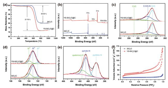
Fig. 4 TGA curves (a) of YS-SiO<sub>x</sub>/C@C and SiO<sub>x</sub>/C, XPS survey spectra (b), high-resolution C1s (c) and Si2p (d) spectra of YS-SiO<sub>x</sub>/C@C and SiO<sub>x</sub>/C, N1s (e) spectrum of YS-SiO<sub>x</sub>/C@C, and N<sub>2</sub> adsorption/desorption isotherms (f) of YS-SiO<sub>x</sub>/C@C and SiO<sub>x</sub>/C.
