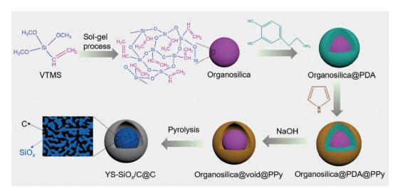
Fig. 1 Schematic illustration of the construction of YS-SiO<sub>x</sub>/C@C composites.
