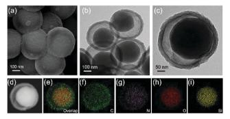
Fig. 3 SEM (a) and TEM (b and c) images of YS-SiO<sub>x</sub>/C@C, and the highangle annular dark field (HAADF) image (d) and its corresponding EDS mapping images (e-i).
