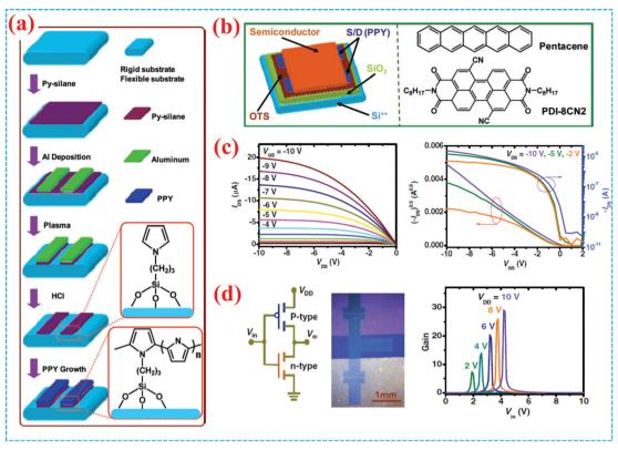
Fig. 9 (a) Schematic patterning process and molecular structure of surface-grafting PPY. (b) Schematic diagram of the OFET and molecular structure of organic semiconductors. (c) Output and transfer curves of the pentacene OFET. (d) Inverters with patterned PPY electrodes and their gain characteristics.<sup>22</sup> Copyright 2012, Wiley-VCH.
