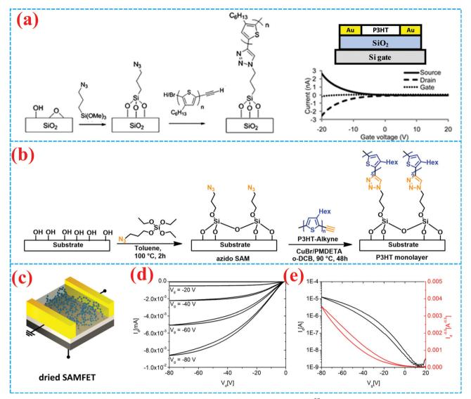
Fig. 13 (a) Synthetic scheme of poly(3-hexylthiophene) brushes and the bottom-contact FET.<sup>58</sup> Copyright 2010, Royal Society of Chemistry. (b) Synthetic scheme of the P3HT monolayer on the substrate. (c) Structure of a SAM-based organic field-effect transistor and (d) output and (e) transfer curves of the grafted SAM dried from chloroform.<sup>59</sup> Copyright 2018, American Chemical Society.
