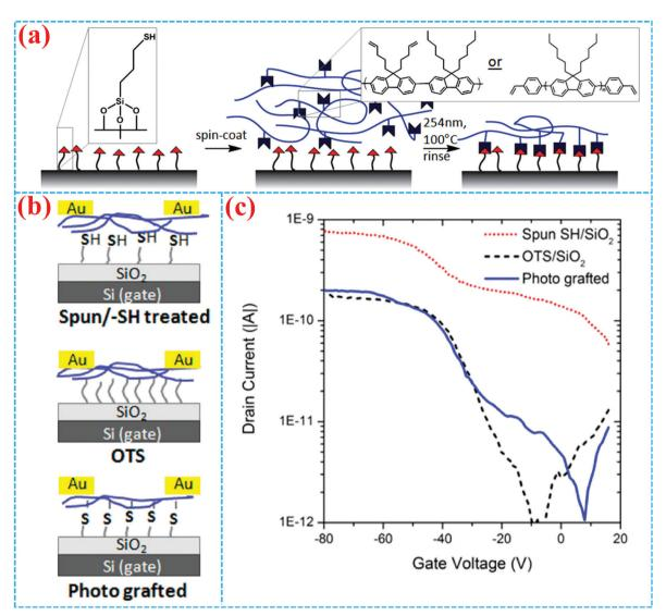
Fig. 14 (a) Synthetic scheme of the surface grafted pPF film. (b) Schematic diagram of pPF OFETs using spun on thiol-functionalized, OTS-treated and photo grafted Si/SiO<sub>2</sub> and their transfer curves. <sup>9</sup> Copyright 2014, American Chemical Society.
