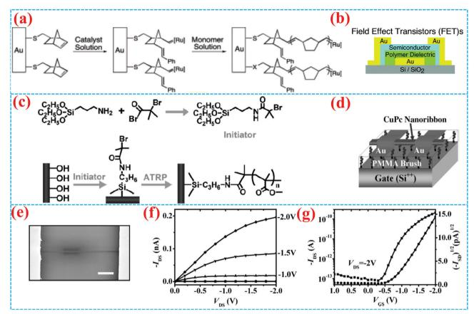
Fig. 3 (a) Construction of the polymer dielectric layer in FETs. (b) Synthetic route for an SI-ROMP polymer dielectric layer on the Au electrode.<sup>54</sup> Copyright 2004, American Chemical Society. (c) Schematic diagram of a CuPc single crystalline nanoribbon OFET with PMMA brush dielectric. (d) Synthetic route for a PMMA brush. (e) SEM image of the CuPc OFET and (f) its output and (g) transfer curves (V<sub>DS</sub> = 2 V) of the OFET. 6 Copyright 2009, Wiley-VCH.
