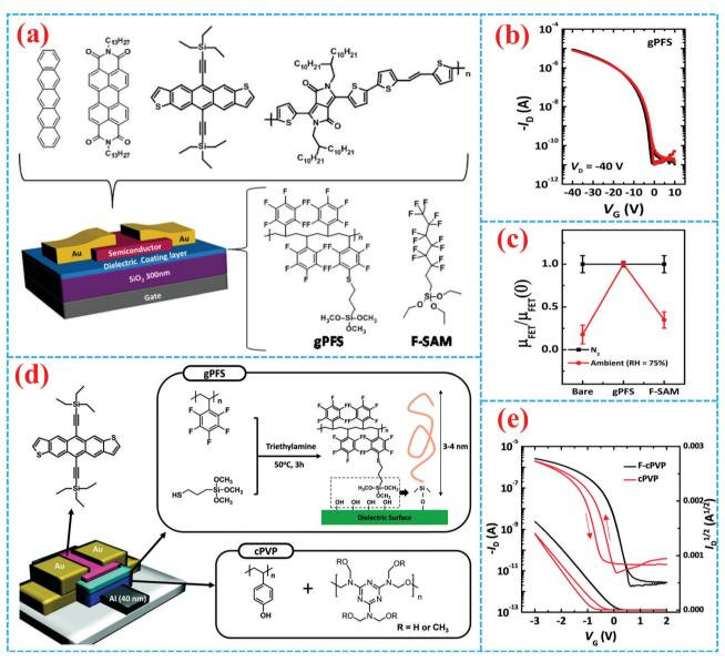
Fig. 7 (a) Representative molecular structure of OFETs based on gPFS and F-SAM. (b) Transfer curves of pentacene OFETs in  $N_2$  (black line) and ambient conditions with a relative humidity of 75% (red line) and (c) the resultant  $\mu_{\text{FET}}$  values. Topyright 2014, American Chemical Society. (d) Schematic diagram of TES-ADT OFET based on gPFS and cPVP dielectric layers and (e) transfer characteristics. 70 Copyright 2015, Royal Society of Chemistry.
