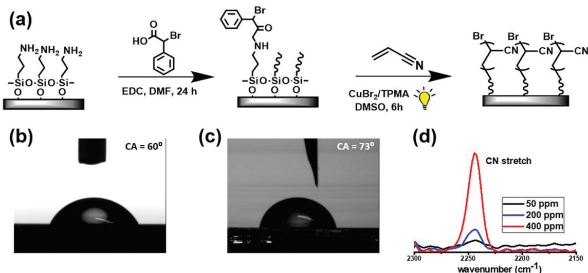
**Fig. 2** (a) Schematic illustration of the synthetic route to PAN brushes by photoinduced SI-ATRP; water contact angle before (b) and after (c) coupling BPAA to the APTES-modified silicon wafer; (d) FT-IR spectra of the surface after SI-ATRP with different catalyst loadings.
