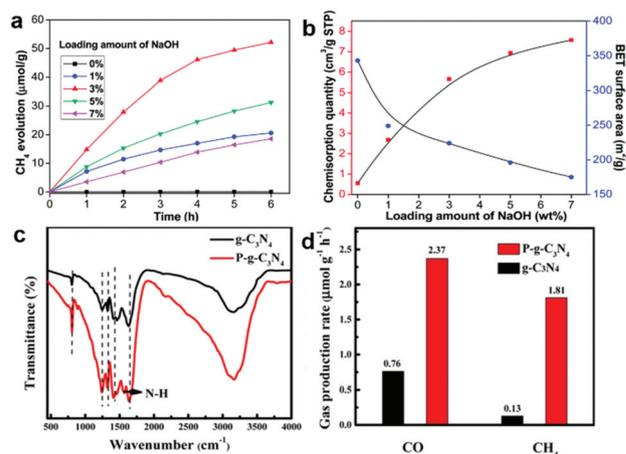
**Fig. 6** (a) Time dependence of CH<sub>4</sub> evolution. (b) Cumulative CO<sub>2</sub> pulse chemisorption quantity and BET surface area of NaOH-TiO<sub>2</sub> composites. Reproduced with permission from ref. 55, copyright 2014 Royal Society of Chemistry. (c) FT-IR spectra and (d) CO and CH<sub>4</sub> yield. Reproduced with permission from ref. 44, copyright 2018 American Chemical Society.
