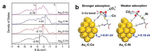
**Fig. 10** (a) Projected density of states (PDOS) of the d-orbitals of surface atoms for Au<sub>c</sub>-C-Fe, Au<sub>c</sub>-C-Co, Au<sub>c</sub>-C-Ni, and Au<sub>c</sub>-C-Cu. (b) Models for CO<sub>2</sub> adsorption on the Au<sub>c</sub>-C-Co surface (left) and Au<sub>c</sub>-C-Ni surface (right). Reproduced with permission from ref. 82, copyright 2018 American Chemical Society.
