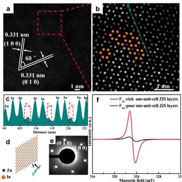
**Fig. 4** Characterization of V<sub>Zn</sub>-rich one-unit-cell ZnIn<sub>2</sub>S<sub>4</sub> (ZIS) layers obtained at 200 °C. HAADF-STEM images (a, b) and intensity profile (c) corresponding to the dark cyan arrow in panel b. The corresponding crystal structures (d) and SAED patterns (e). (f) EPR spectra of V<sub>Zn</sub>-rich and V<sub>Zn</sub>-poor one-unit-cell ZIS layers. Reproduced with permission from ref. 35, copyright 2017 American Chemical Society.
