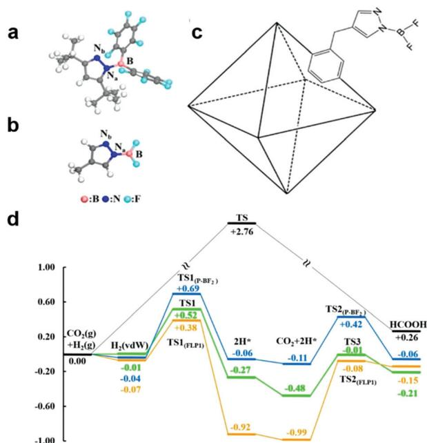
**Fig. 7** Structure of frustrated Lewis pairs (FLP<sub>1</sub>) (a) and P-BF<sub>2</sub> (b). (c) Schematic of a UiO-66 primitive cell functionalized with P-BF<sub>2</sub>. (d) Relative potential energy surfaces for gas phase CO<sub>2</sub> hydrogenation without a catalyst (black), catalyzed by FLP<sub>1</sub> (orange), catalyzed by P-BF<sub>2</sub> (blue), and catalyzed by UiO-66-P-BF<sub>2</sub> (green). Reproduced with permission from ref. 59, copyright 2015 American Chemical Society.
