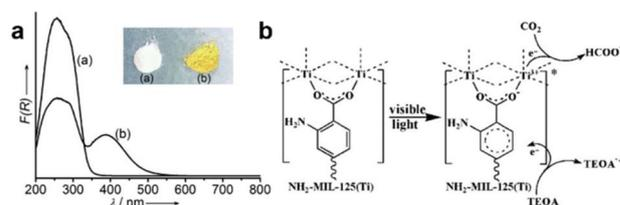
Fig. 11 (a) UV-vis spectra of MIL-125(Ti) and  $\text{NH}_2\text{-MIL-125}(\text{Ti})$ . (b) Proposed mechanism of  $\text{CO}_2$  reduction over  $\text{NH}_2\text{-MIL-125}(\text{Ti})$  under visible light irradiation. Reproduced with permission from ref. 100, copyright 2012 John Wiley and Sons.
