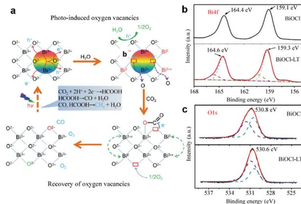
**Fig. 3** (a) Possible reaction pathways for CO<sub>2</sub> photoreduction with H<sub>2</sub>O on BiOCl nanoplates. (b) XPS spectra of the Bi<sub>4f</sub> region and (c) the O<sub>1s</sub> region for BiOCl and BiOCl-LT nanoplates. Reproduced with permission from ref. 31, copyright 2015 Springer.
