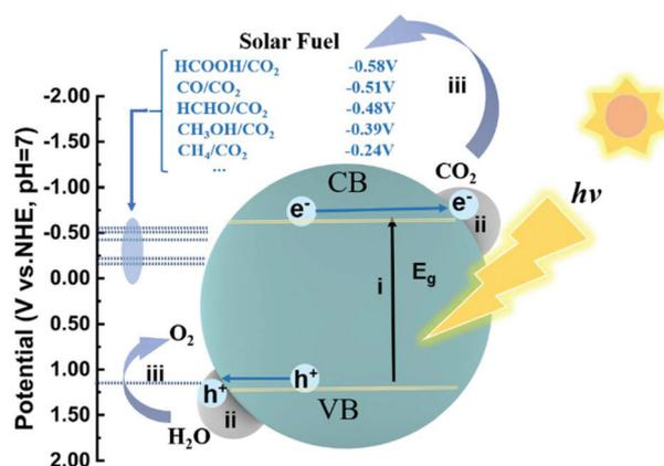
Fig. 1 Schematic illustration of the overall process for photocatalytic CO<sub>2</sub> reduction with H<sub>2</sub>O over a semiconductor photocatalyst. The dotted lines indicate the thermodynamic potentials for water oxidation into O<sub>2</sub> and CO<sub>2</sub> reduction into CH<sub>4</sub>, CH<sub>3</sub>OH, HCHO, CO and HCOOH, respectively. The numbers i, ii and iii represent the three critical steps in photocatalytic CO<sub>2</sub> reduction.
