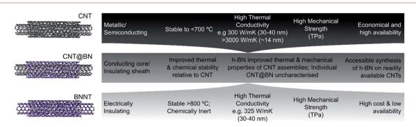
Fig. 9 A comparison of the main properties and availability of CNT@BNs, pure CNTs and BNNTs. See previous reviews for more detailed comparisons of CNTs versus BNNTs.<sup>65–67</sup>
