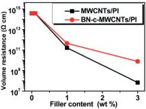
**Fig. 14** (a) Thermal conductivity and (b) volume resistivity of polyimide matrix composites with either raw MWCNT filler or h-BN coated MWCNT filler at three different weight percentages. Reproduced from ref. 34 with permission from the Royal Society of Chemistry.
