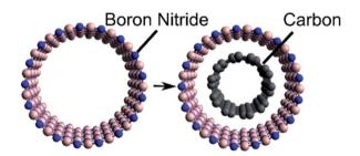
Method B: Depositing h-BN onto CNT
