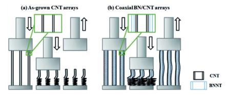
Fig. 12 Illustration that coating of h-BN onto VA-MWCNTs changed mechanical response to compression. (a) Pristine MWCNTs underwent plastic deformation upon compression. (b) BN coated MWCNTs with 3-walls of BN exhibited elastic recovery. Reproduced from ref. 21 with permission from the Royal Society of Chemistry.
