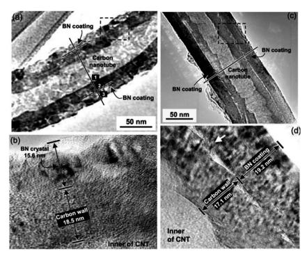
Fig. 7 (a and b) TEM and HRTEM images of rough, polycrystalline h-BN coating formed on pyrolytically stripped MWCNT. (c and d) TEM and HRTEM images of smooth, crystalline h-BN coating formed on heated treated (3000 °C) MWCNT. Surface crystallinity of the MWCNT influences the h-BN coating crystallinity. Reproduced with permission from ref. 29. Copyright 2004, The American Ceramic Society.
