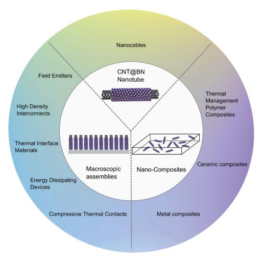
Fig. 10 Summary of some potential applications of CNT@BN heteronanotubes as individual nanotubes, macroscopcic arrangements or nanocomposites
