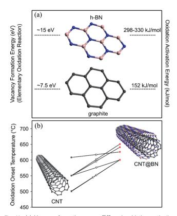
Fig. 11 (a) Vacancy formation energy<sup>78,83</sup> and oxidation activation energy<sup>52</sup> of h-BN vs. graphitic carbon, justifying why h-BN is more oxidatively stable at high temperatures that graphitic carbon. (b) Compiled oxidation onset temperature values from studies that reported TGA results on CNTs prior to h-BN coating and after h-BN coating,<sup>21,27,30,31,39,50</sup> suggesting that h-BN was effective at improving oxidation resistance.
