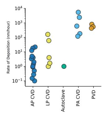
Fig. 5 Calculated h-BN deposition rate (nm per hour) amongst the various methods of CVD (atmospheric pressure, 21,27-35 low pressure, 20,36-38 autoclave, 39 plasma assisted 40,41) and PVD.41 Rates are shown on a log 10 scale.
