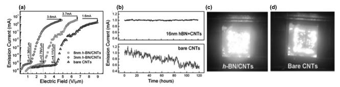
Fig. 15 (a) Graph showing that the 3 nm h-BN coating on MWCNTs reduced the emission turn on field in comparison to pristine MWCNTs and MWCNTs coated with 8 nm BN. (b) By introducing a h-BN coating, the emission current stability was significantly enhanced in comparison to bare CNTs. (c) Emission images for 2 mm  $\times$  2 mm array of VA-MWCNTs coated with 3 nm h-BN compared to (d) pristine MWCNTs. Reproduced with permission from ref. 36. Copyright 2015, Wiley-VHC.
