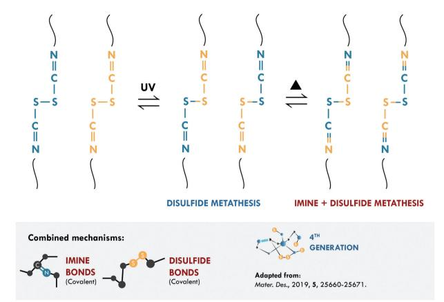
Fig. 9 Imine and disulfide metathesis in PU. $^{187}$   $\odot$ 2019. Adapted with permission from Elsevier.
