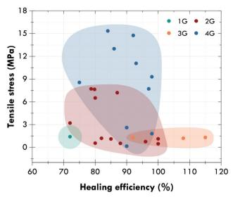
Fig. 12 Ashby diagram of the four generations of self-healing elastomers.
