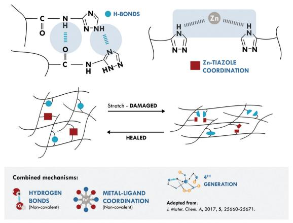
Fig. 7 Combination between hydrogen bonds and metal-ligand coordination in IR.<sup>172</sup> ©2017. Adapted with permission from the Royal Society of Chemistry.
