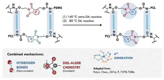
Fig. 11 Combination between DA chemistry and hydrogen bonds in PDMS-DA-PU.<sup>200</sup> ©2016. Adapted with permission from the Royal Society of Chemistry.
