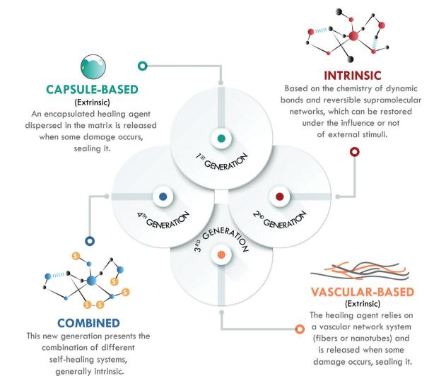
Fig. 2 Generations of self-healing materials according to the healing mechanism involved.
