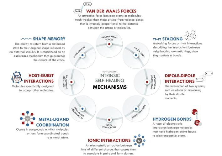
Fig. 5 Non-covalent intrinsic self-healing mechanisms
