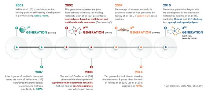
Fig. 3 Timeline of generations in self-healing polymers.
