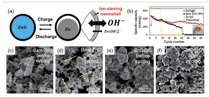
Fig. 3 (a) Schematic showing ZnO nanoparticles coated with an ion-sieving carbon nanoshell; (b) specific capacity and coulombic efficiency of bare ZnO, ZnO@C, and bulk Zn foil anodes during discharge; (c and d) SEM images of the bare ZnO anode (c) before and (d) after cycling; (e and f) SEM images of the ZnO@C anode (e) before and (f) after cycling, ref. 65, copyright@ 2018 WILEY-VCH Verlag GmbH & Co. KGaA, Weinheim.
