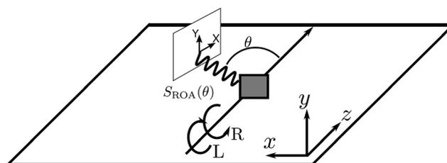
Fig. 1 The ROA measurement scheme. Left and right circularly polarized X-ray pulses propagating along the *z* direction generate two Raman signals which are recorded as a function of the scattering angle. Their small difference constitutes the ROA signal, eqn (9). The detector polarization basis by *X* and *Y* provides an extra degree of freedom for the measurement.
