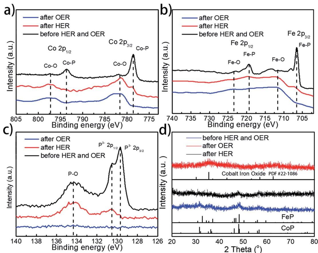
Fig. 7 High-resolution (a) Co 2p, (b) Fe 2p, and (c) P 2p XPS spectra of the as-prepared, post-HER and post-OER  $\text{Co}_{0.6}\text{Fe}_{0.4}\text{P-1.125}$  catalysts; (d) XRD patterns of the as-prepared, post-HER and post-OER  $\text{Co}_{0.6}\text{Fe}_{0.4}\text{P-1.125}$  catalysts.
