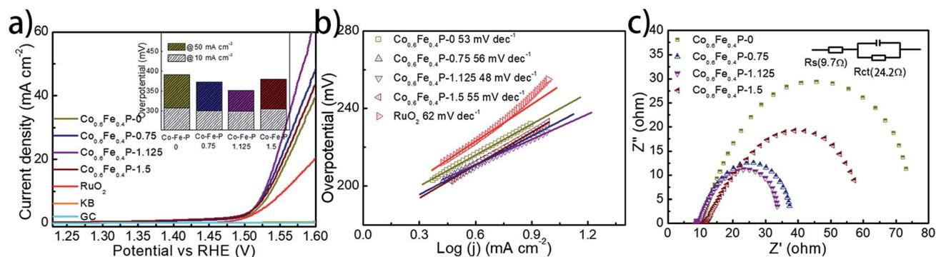
Fig. 5 (a) Polarization curves of  $\text{Co}_{0.6}\text{Fe}_{0.4}\text{P}$  and control samples for the OER in 1.0 M KOH (inset: the column diagram of OER activities for all  $\text{Co}_{0.6}\text{Fe}_{0.4}\text{P}$  catalysts); (b) the corresponding Tafel plots of all the  $\text{Co}_{0.6}\text{Fe}_{0.4}\text{P}$  catalysts and  $\text{RuO}_2$ ; (c) Nyquist plots of all  $\text{Co}_{0.6}\text{Fe}_{0.4}\text{P}$  catalysts at  $-1.53 \text{ V}$  over the frequency range from 100 000 to 0.01 Hz.
