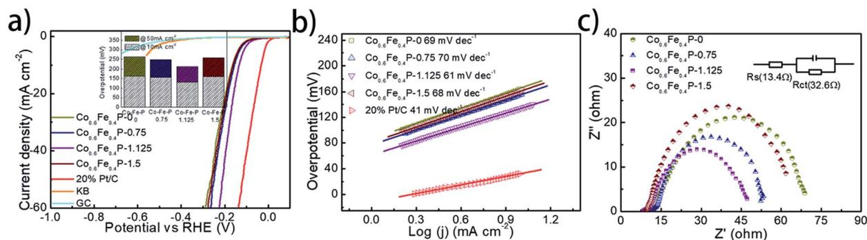
Fig. 4 (a) Polarization curves of  $\text{Co}_{0.6}\text{Fe}_{0.4}\text{P}$  and control samples for the HER in 1.0 M KOH (inset: the column diagram of HER activities for all  $\text{Co}_{0.6}\text{Fe}_{0.4}\text{P}$  catalysts); (b) the corresponding Tafel plots of all the  $\text{Co}_{0.6}\text{Fe}_{0.4}\text{P}$  catalysts and 20% Pt/C; (c) Nyquist plots of all  $\text{Co}_{0.6}\text{Fe}_{0.4}\text{P}$  catalysts at  $-0.15 \text{ V}$  over the frequency range from 100 000 to 0.01 Hz.
