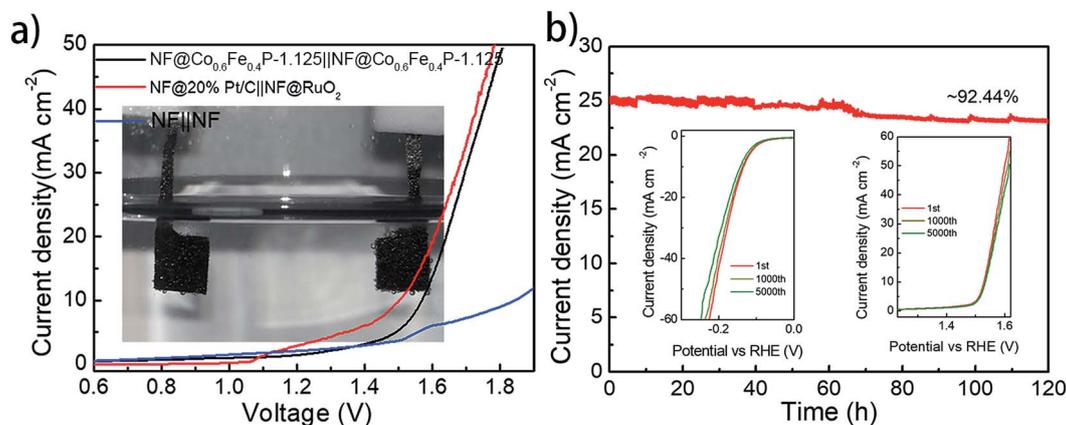
Fig. 6 (a) The overall water splitting performance of the  $\text{Co}_{0.6}\text{Fe}_{0.4}\text{P}$ -1.125 and Pt/C|| $\text{RuO}_2$  couple in 1.0 M KOH (inset: photo of the overall water splitting reaction in a two-electrode configuration); (b) the catalytic stability of the  $\text{Co}_{0.6}\text{Fe}_{0.4}\text{P}$ -1.125 for overall water splitting in 1.0 M KOH (inset: the durability of  $\text{Co}_{0.6}\text{Fe}_{0.4}\text{P}$ -1.125 for the HER and OER after 1000 and 5000 CV cycles).
