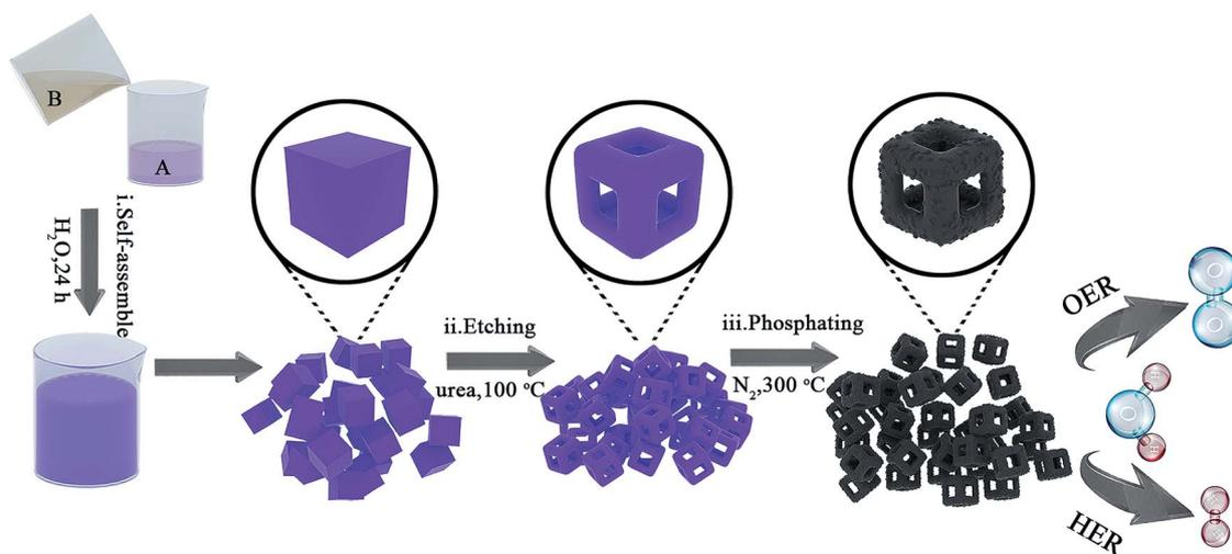
Fig. 1 Schematic illustration of the preparation of the nanoframes composed of Co<sub>0.6</sub>Fe<sub>0.4</sub>P NPs coated with the carbon matrix. (i) Self-assembly of Co–Fe PBA; (ii) etching of the Co–Fe PBA to produce nanocages; (iii) phosphidation of the Co–Fe PBA nanocages to obtain subsequent Co<sub>0.6</sub>Fe<sub>0.4</sub>P NPs coated with the carbon matrix.
