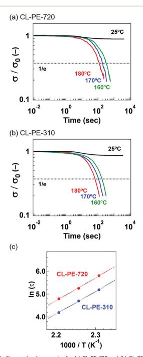
Fig. 4 Stress-relaxation spectra for (a) CL-PE-720 and (b) CL-PE-310, where the stress  $(\sigma)$  is normalized by the initial stress  $(\sigma_0)$ . The dotted lines in (a) and (b) indicate the point at  $\sigma/\sigma_0=1/e$  (=0.3679). (c) Arrhenius plots of  $\tau$  as a function of inverse temperatures.
