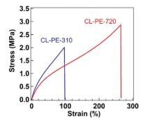
Fig. 2 Stress-strain curves for CL-PE-720 (red) and CL-PE-310 (blue).
