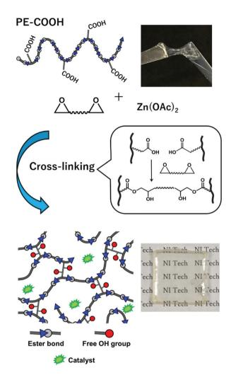
**Fig. 1** Schematic of the present molecular design. Free OH groups are generated by the epoxy-opening reaction with COOH groups in PE-COOH during the cross-linking reaction. The pictures of samples before and after cross-linking are also shown.
