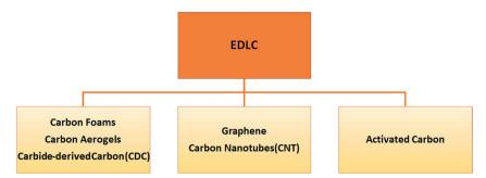
Fig. 2 Classification of electrochemical double layer capacitors (EDLCs)
