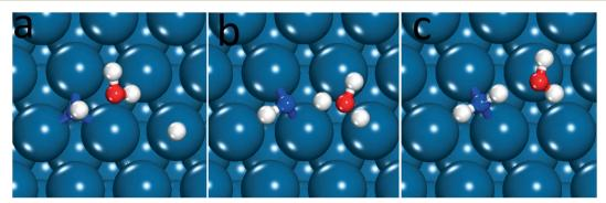
Fig. 4 Reaction path for NH\* hydrogenation on the Pt(111) surface, (a) initial state, (b) transition state and (c) final state.
