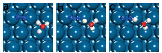
Fig. 1 Equilibrium and transition states for N2 reduction to N2H\* on Pt(111), (a) initial state, (b) transition state and (c) final state.
