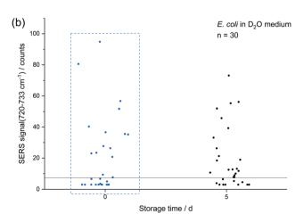
Fig. 5 (a) SERS signal at around 733 cm $^{-1}$  of *E. coli* with and without 25% D<sub>2</sub>O addition plotted against Raman shift (bars: 1 s); (b) SERS intensity of *E. coli* with 25% addition of D<sub>2</sub>O after 0 and 5 d storage. Note that the data at day 0 in the blue box of panel (b) corresponds to the deuterium data in the blue box of panel (a).
