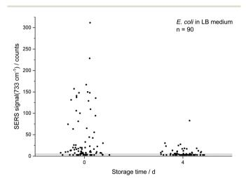
**Fig. 2** Decreasing absolute SERS intensity at 733 cm<sup>-1</sup> of single *E. coli* (LB medium) cells which were cultured to the stationary phase and either directly subjected to *in situ* AgNP synthesis or first stored for 4 d. Values are scattered on the abscissa for better readability.
