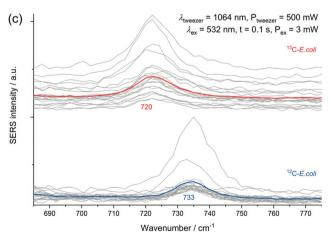
Fig. 6 (a) Continuously acquired spectra of an AgNP@E. coli particle inside the laser focus. (b) Microscopic image during sorting by optical tweezing with an AgNP@E. coli particle inside the laser focus. (c) Consecutive SERS spectra of <sup>13</sup>C-E. coli (red mean spectrum) and <sup>12</sup>C-E. coli (blue mean spectrum) inside of the same sample with activated optical tweezer laser. Associated spectra are shifted on the ordinate for a better visualization.
