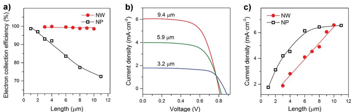
Fig. 4 Performance of the rutile  $\text{TiO}_2$  NW and NP-based solar cells. (a) Dependence of the electron collection efficiency on the NW length and NP-film thickness. (b) Comparison of the current density–voltage characteristics of the NW-based cells under AM 1.5 illumination. (c) Dependence of current density on the NW length and NP-film thickness.
