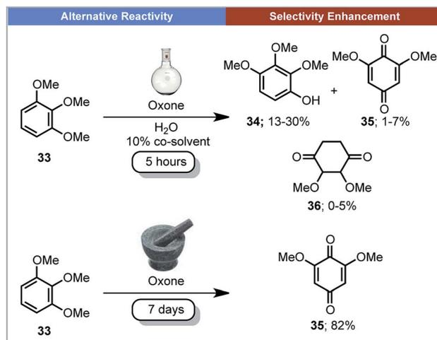
Scheme 11 Oxidation of lignin-like methoxylated aromatics; Anastas, Crabtree, Hazari and co-workers.<sup>64</sup>
