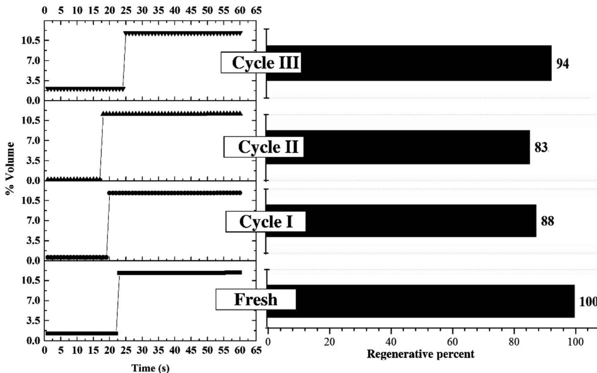
Fig. 10 Effect of regeneration cycle on CO<sub>2</sub> sorption capacity.
