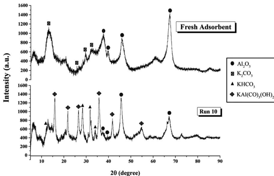
Fig. 9 XRD pattern of sorbent before and after CO<sub>2</sub> sorption.<sup>32,33,40</sup>
