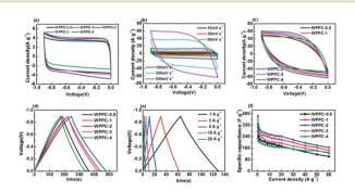
Fig. 5 Capacitive performance of the WPPCs in the KOH electrolyte: (a) CV curves of the WPPCs at 30 mV s $^{-1}$ , (b) CV curves of the WPPC-2 at 10 $^{-500}$  mV s $^{-1}$ , (c) CV curves of the WPPCs at 500 mV s $^{-1}$ , (d) GCD curves of WPPCs at 0.3 A g $^{-1}$ , (e) GCD curves of the WPPC-2 at 1 $^{-20}$  A g $^{-1}$ , (f) specific capacitances of WPPCs at different discharge current densities.
