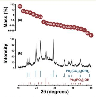
Fig. 3 (a) Median mass fraction by element for triplicate scale samples representing an LSL recovered from system A. (b) XRD analysis was consistent with the presence of hydrocerussite, Pb<sub>3</sub>(CO<sub>3</sub>)<sub>2</sub>(OH)<sub>2</sub>, and hydroxypyromorphite, Pb<sub>5</sub>(PO<sub>4</sub>)<sub>3</sub>OH.
