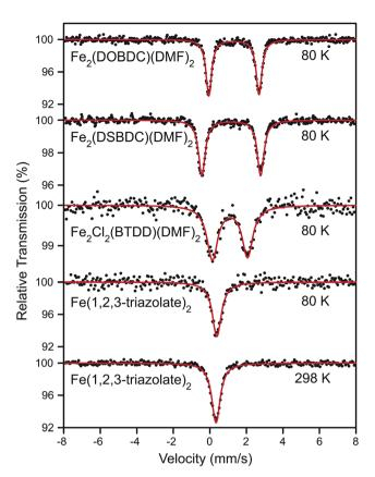
Fig. 4 <sup>57</sup>Fe Mössbauer spectra of Fe<sub>2</sub>(DOBDC)(DMF)<sub>2</sub>, Fe<sub>2</sub>-(DSBDC)(DMF)<sub>2</sub>, and Fe<sub>2</sub>Cl<sub>2</sub>(BTDD)(DMF)<sub>2</sub> at 80 K as well as Fe(1,2,3triazolate)<sub>2</sub> at 80 and 298 K. All samples were kept in N<sub>2</sub> atmosphere. Black dots represent experimental data, and red curves represent Lorentzian fitting curves.
