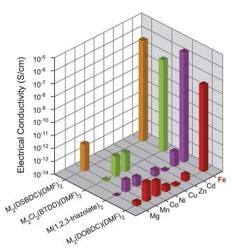
2 Electrical conductivity in M2(DOBDC)(DMF)2. (DSBDC)(DMF)<sub>2</sub>, M<sub>2</sub>Cl<sub>2</sub>(BTDD)(DMF)<sub>2</sub>, and M(1,2,3-triazolate)<sub>2</sub> measured at 300 K, in N<sub>2</sub> atmosphere, and in the dark.
