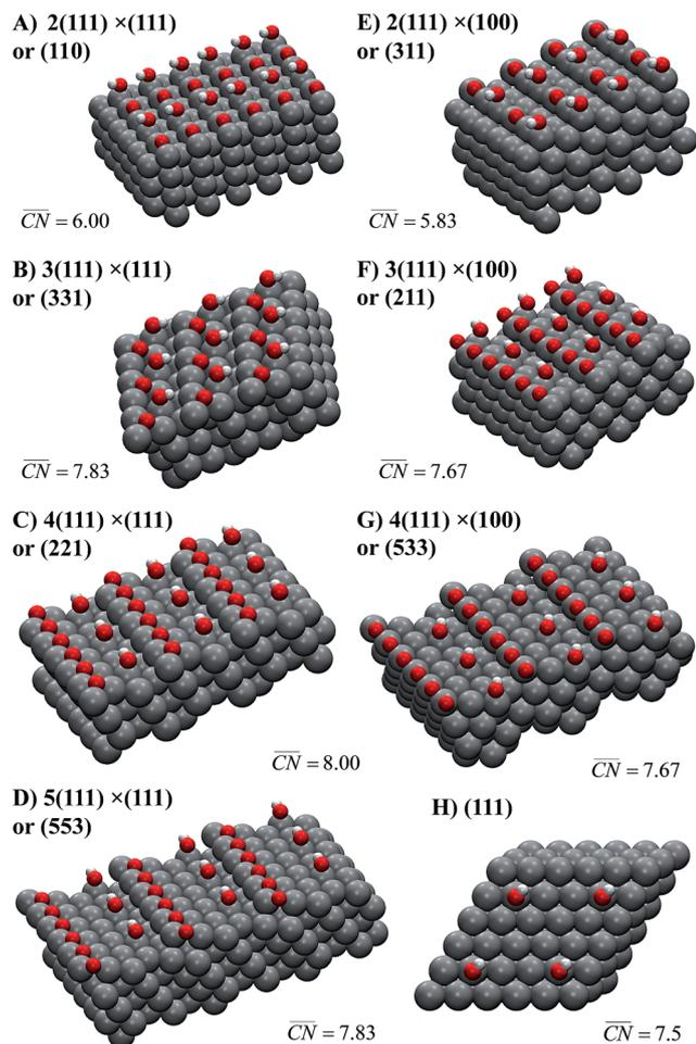
Fig. 2 Most active sites on Pt single-crystal surfaces for the ORR. \*OH sits at the active sites, which are located in all cases at the bottom of the steps ( $\overline{CN}$  is provided in each case, see Section S2 in the ESI† for details of its assessment). The Miller indices of the surfaces are provided together with the length of their (111) terraces and step types, namely (111)-like (left) or (100)-like (right). In all cases, the step edges are covered with \*O.
