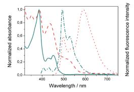
Fig. 4 Normalized absorbance of compound 1 (—) and 2 (— —) in  $CH_2Cl_2$  and corresponding normalized fluorescence emission spectra upon excitation at 385 (— · —) and 440 (····) nm, respectively.
