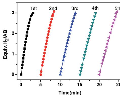
Fig. 5 The plots of volume of H<sub>2</sub> vs. time for hydrolysis of AB catalyzed by the 5% Co/CTF-1 catalyst during a five-cycle reusability test.
