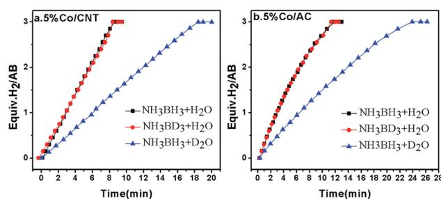
Fig. 1 Hydrogen evolution from NH<sub>3</sub>BH<sub>3</sub> in H<sub>2</sub>O (black), NH<sub>3</sub>BD<sub>3</sub> in H<sub>2</sub>O (red), and NH<sub>3</sub>BH<sub>3</sub> in D<sub>2</sub>O (blue) catalyzed by 5% Co/CNT (left) and 5% Co/AC (right) at room temperature,  $n_{Co} : n_{AB} = 0.05 : 1$ .
