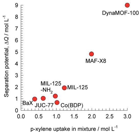
Fig. 10 The separation potential,  $\Delta Q_{(oX+mX+EthBz)/pX}$  for separation of 4-component *o*-xylene/*m*-xylene/*p*-xylene/ethylbenzene mixtures plotted against the volumetric uptake of *p*-xylene. All calculation details and structural information on the various MOFs are provided in the ESI.†
