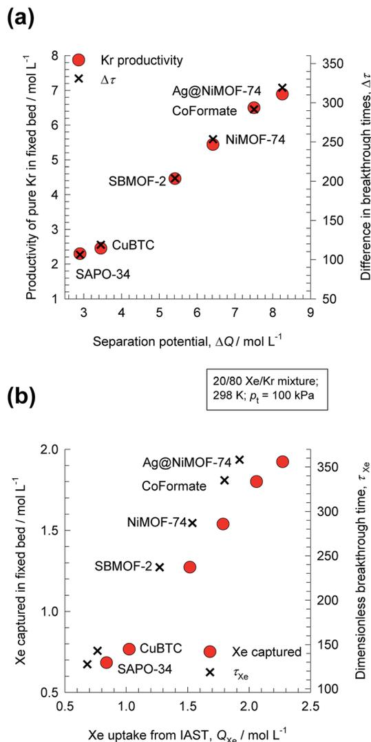
Fig. 4 (a) Plot of pure Kr (containing <1000 ppm Xe) productivity as a function of the separation potential  $\Delta Q_{Kr/Xe} = Q_{Xe} \frac{80}{20} - Q_{Kr}$ , calculated from IAST for six different MOFs at temperature  $T = 298$  K, and total pressure  $p_t = 100$  kPa. (b) Plot of Xe capture capacity in fixed bed as a function of the Xe uptake  $Q_{Xe}$ , calculated from IAST. Also plotted as right y-axes are (a)  $\Delta\tau = \tau_{Xe} - \tau_{Kr}$  and (b)  $\tau_{Xe}$ .
