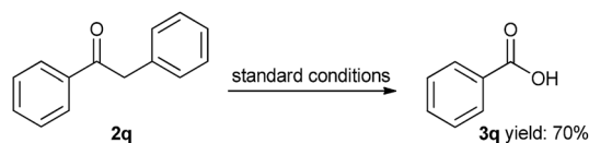
Scheme 2 Oxidative reaction of 2-phenylacetophenone.
