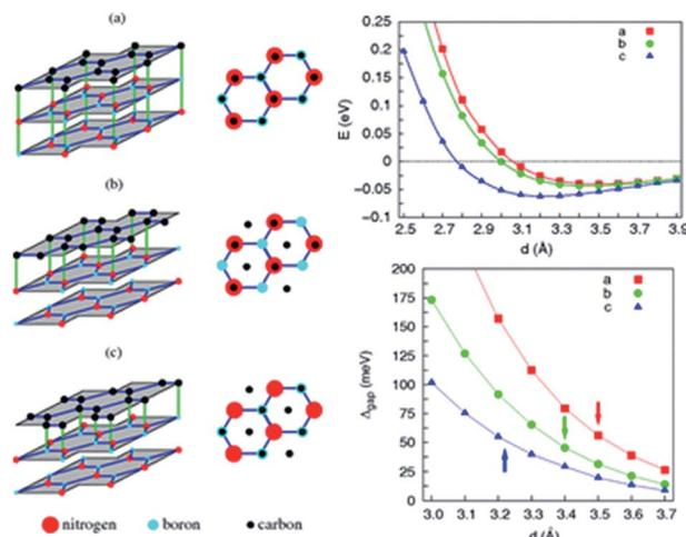
Fig. 34 The three inequivalent orientations of single-layer graphene on a h-BN surface and the total energy  $E$  of graphene on a h-BN surface for the three manners.<sup>71</sup>
