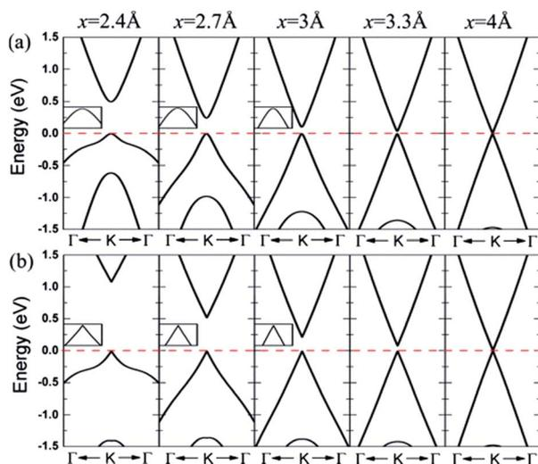
Fig. 21 Band lines near the Fermi level of C/BN HBLs with interlayer distances  $x = 5, 3.3, 3, 2.7,$  and  $2.4 \text{ \AA}$  for (a) configuration II and (b) configuration IV. The Fermi level is set to zero.<sup>166</sup>
