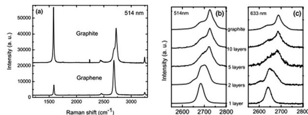
Fig. 11 Raman spectra of ideal graphene and of different layers under different wavelengths.<sup>113</sup>
