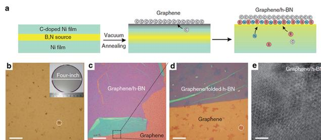
Fig. 31 Growth of graphene/h-BN-stacked heterostructures: schematic illustration and optical images of the as-grown sample on the growth substrates.<sup>188</sup>
