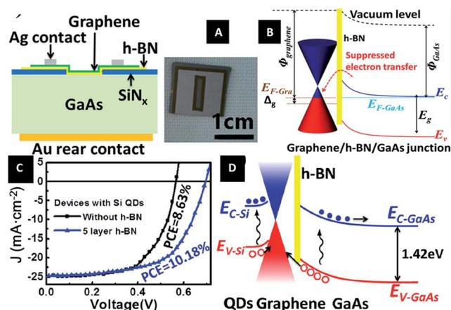
Fig. 41 Graphene/h-BN/GaAs sandwich diode as a solar cell and photodetector. (A) Schematic of the graphene/h-BN/GaAs sandwich device. (B) Electronic band structure of graphene/h-BN/GaAs heterostructure. (C)  $J-V$  curves of solar cells based on graphene/GaAs and graphene/h-BN/GaAs heterostructure with Si QDs introduced photo-induced doping. (D) Electronic band structure of the graphene/h-BN/GaAs solar cell with Si QDs covering on graphene under illumination.<sup>212</sup>
