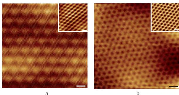
Fig. 33 Real space and Fourier transforms of Moiré patterns with different ratio in (a) and (b).<sup>195</sup>
