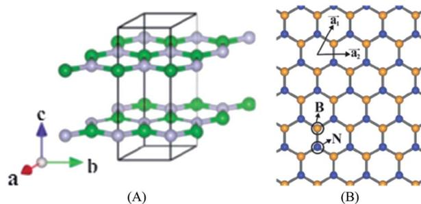
Fig. 12 Structure of h-BN. (A) Stereogram. (B) The 2D floor plan.<sup>118</sup>
