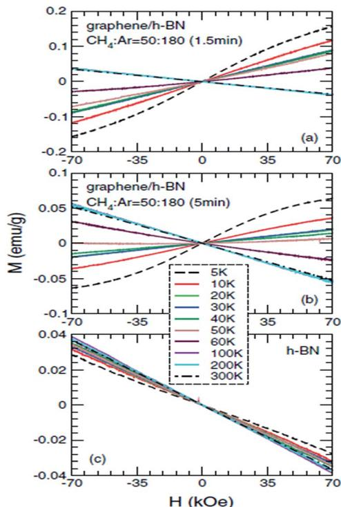
Fig. 36 The measured mass magnetization  $M$  as functions of magnetic fields  $H$  for (a) gra/h-BN sample 1, (b) gra/h-BN sample 2, and (c) h-BN substrate, at different temperatures  $T = 5, 10, 20, 30, 40, 50, 60, 100, 200,$  and  $300$  K.<sup>203</sup>
