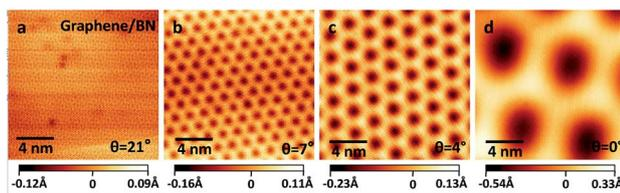
Fig. 19 STM pictures of graphene/h-BN heterostructure with different rotational orientations.<sup>70</sup>
