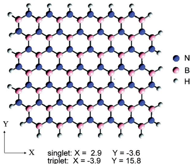
Fig. 2 Flat structure diagram of h-BN. Blue on behalf of nitrogen atoms and pink on behalf of boron atoms, respectively.<sup>34</sup>
