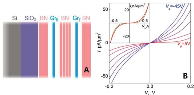
Fig. 38 Schematic of a field-effect tunnelling transistor (A) and (B) tunnelling characteristics for a graphene/h-BN device with  $6 \pm 1$  layers of h-BN as the tunnel barrier.<sup>182</sup>
