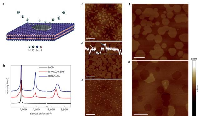
Fig. 30 The method of epitaxial graphene growth and the AFM image.<sup>187</sup>
