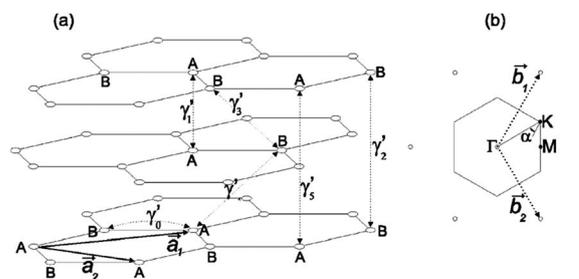
Fig. 4 (a) The relationship between distribution of A and B atoms in the unit cell of graphene. (b) Corresponding Brillouin zone. The Dirac cones are located at the K and M points.<sup>79</sup>
