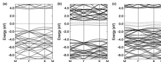
Fig. 17 Calculated band structures of the pristine graphitic-BN with different atoms. (a) with a boron atom (b) and a nitrogen atom (c) substituted by a carbon atom.<sup>148</sup>
