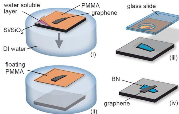
Fig. 24 Schematic of the transfer process to fabricate graphene-on-BN devices.<sup>72</sup>
