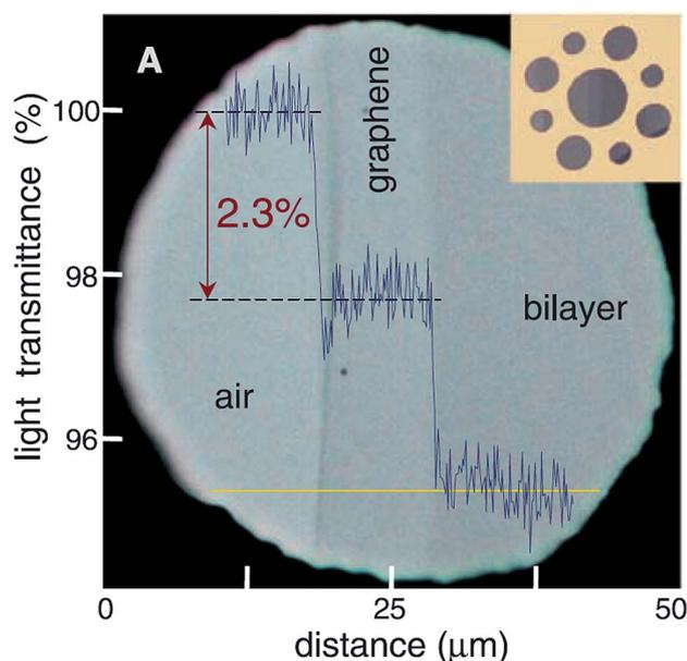
Fig. 8 Looking through one-atom-thick crystals.<sup>95</sup>
