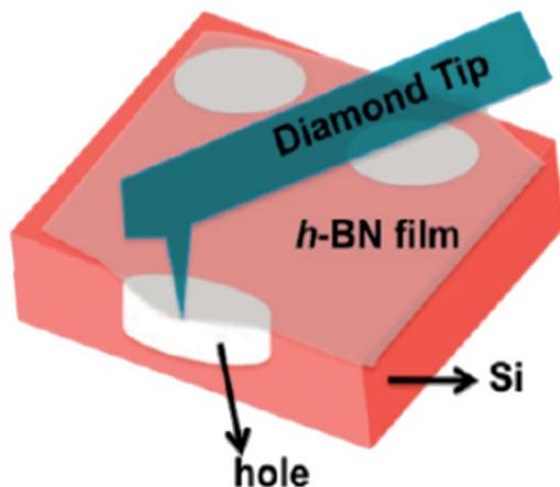
Fig. 15 Schematic of nanoindentation on a suspended h-BN membrane.<sup>133</sup>
