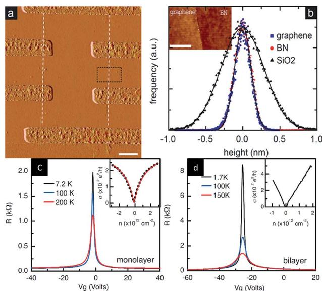
Fig. 37 Graphene/h-BN devices and the test chart. (a) AFM image of graphene/h-BN heterostructure. (b) Histogram of the height distribution measured by AFM for graphene, h-BN and  $\text{SiO}_2$ . Resistance versus applied gate voltage for monolayer graphene (c) and bilayer graphene (d) on h-BN.<sup>204</sup>
