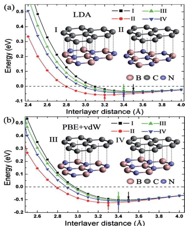
Fig. 20 BE per unit cell of graphene/h-BN with different stacking manners.<sup>166</sup>
