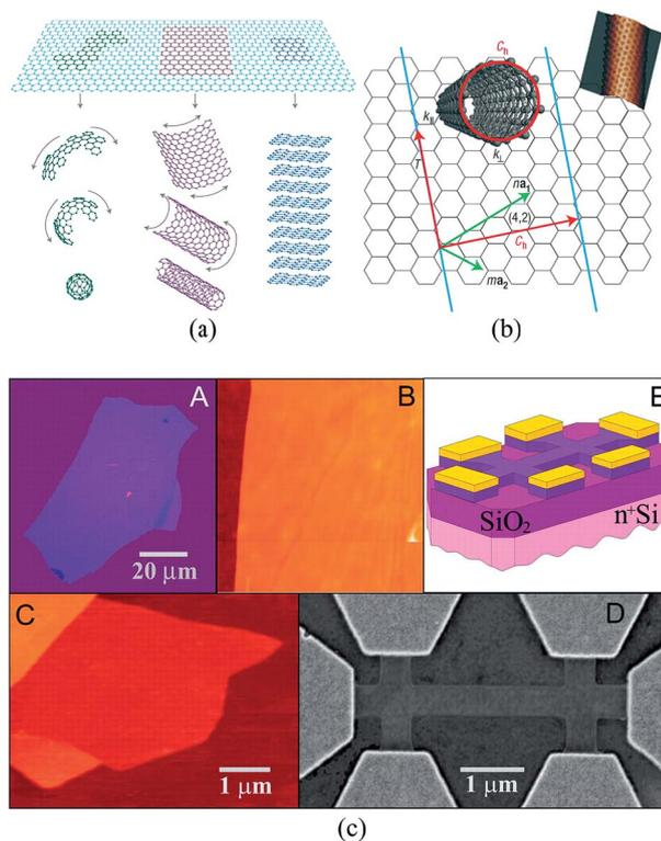
**Fig. 1** (a) The basic unit of the other C material – graphene.<sup>1</sup> (b) The relational graph between graphene and carbon nanotubes.<sup>7</sup> (c) Graphene film and devices (flow chart of graphene prepared by mechanical stripping method from A to E).<sup>3</sup>
