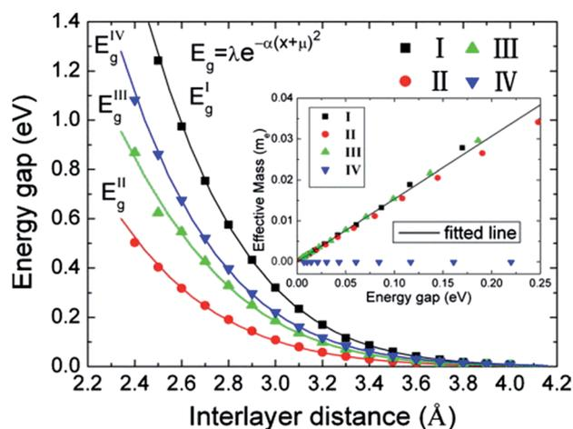
Fig. 22 Variation in the energy gap of HBLs as a function of interlayer spacing. The inset shows the variation of the effective masses vs. the band gap.<sup>166</sup>
