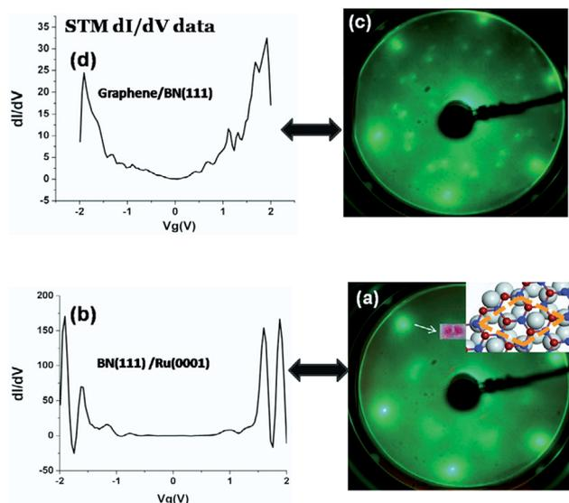
Fig. 28 LEED and STM  $dI/dV$  data for BN monolayer and graphene/h-BN heterojunction grown on Ru(0001).<sup>162</sup>
