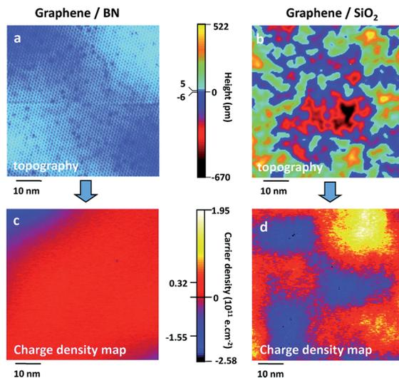
Fig. 3 Comparison of the topography and charge density for graphene/BN vs. graphene/SiO<sub>2</sub>.<sup>73</sup>
