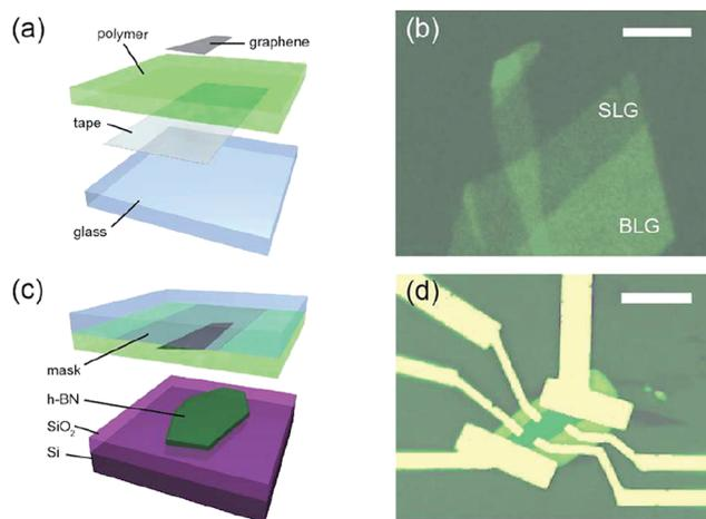
Fig. 26 Dry preparation of graphene/h-BN as a schematic and sample image: (a) schematic of the transfer mask. (b) SLG and BLG areas on the mask, the scale bar equals 5  $\mu\text{m}$ . (c) Graphene alignment and transfer to a h-BN crystal. (d) Graphene flake in a Hall bar geometry on h-BN.<sup>170</sup>
