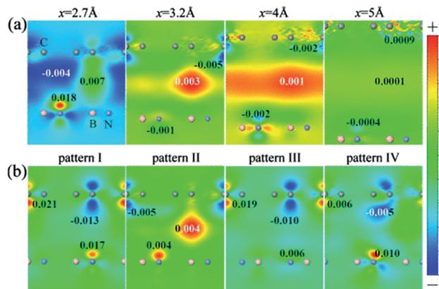
Fig. 23 Contour plots of the charge density difference (a) for stacking pattern I at the interlayer distances  $x = 2.7, 3.2, 4$  and  $5 \text{ \AA}$ , respectively, and (b) for the four stacking patterns (I–IV) at the interlayer distance  $x = 3 \text{ \AA}$ .<sup>198</sup>
