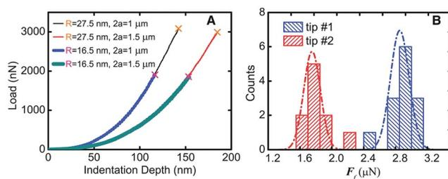
Fig. 6 Fracture test results (A) the test line corresponding to different film diameters and tip radius. (B) Histogram and Gauss distribution of two kinds of fracture forces.<sup>9</sup>
