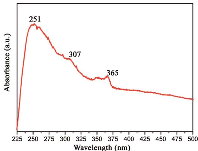
Fig. 16 UV-vis optical absorption spectra of BN.<sup>131</sup>
