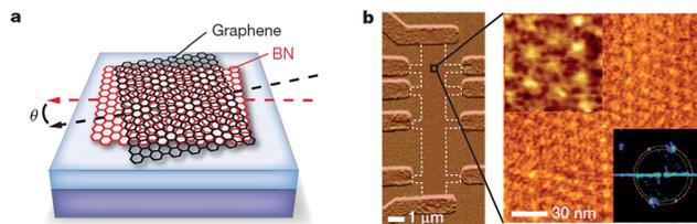
Fig. 29 Moire' superlattice of graphene/h-BN. (a) The schematic diagram of moiré pattern for graphene on h-BN. (b) AFM image of a multiterminal Hall bar and a high-resolution image of a magnified region.<sup>185</sup>
