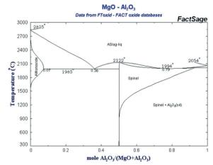
Fig. 14 Phase diagram of magnesium aluminates.
