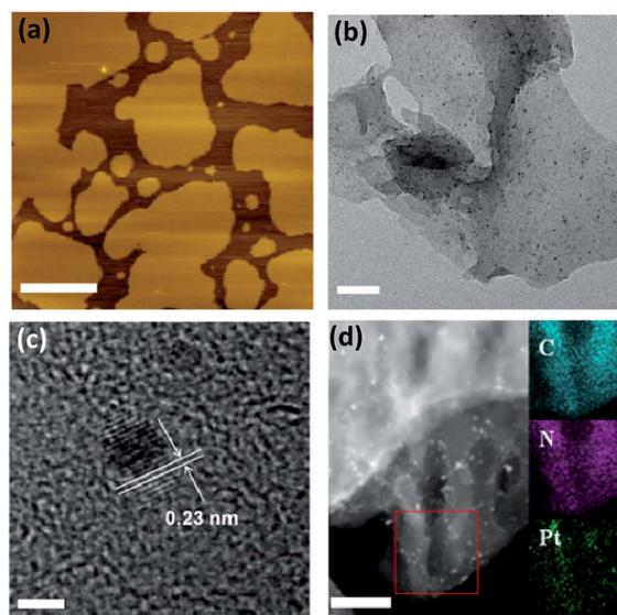
**Fig. 2** (a) AFM image of the  $g\text{-C}_3\text{N}_4$  polymers with Pt deposited *in situ*. (b) TEM image of the  $g\text{-C}_3\text{N}_4$  polymers with Pt deposited *in situ*. (c) HR-TEM image of the  $g\text{-C}_3\text{N}_4$  polymers with Pt deposited *in situ*. (d) STEM images of the  $g\text{-C}_3\text{N}_4$  polymers with Pt deposited *in situ*. Scale bar for a, b, c and d is 50 nm, 100 nm, 2 nm and 50 nm, respectively.
