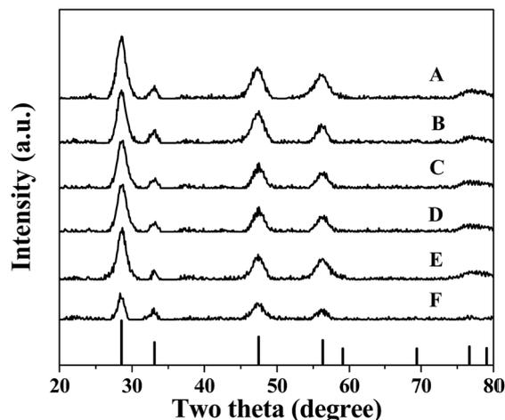
Fig. 5 XRD patterns of (A) Cu–CeO<sub>2</sub>–Pt; (B) Cu<sub>0.66</sub>Co<sub>0.34</sub>–CeO<sub>2</sub>–Pt; (C) Cu<sub>0.50</sub>Co<sub>0.50</sub>–CeO<sub>2</sub>–Pt; (D) Cu<sub>0.34</sub>Co<sub>0.66</sub>–CeO<sub>2</sub>–Pt; (E) Co–CeO<sub>2</sub>–Pt; (F) CeO<sub>2</sub>–Pt.
