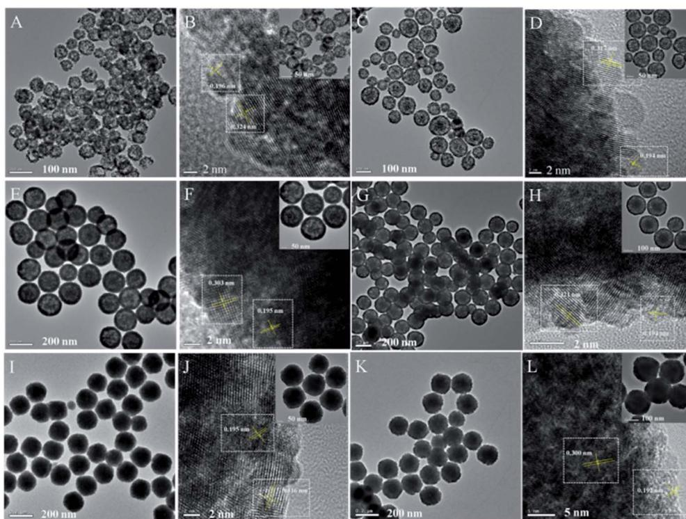
Fig. 3 TEM images of (A) and (B) Cu–CeO<sub>2</sub>–Pt; (C) and (D) Cu<sub>0.66</sub>Co<sub>0.34</sub>–CeO<sub>2</sub>–Pt; (E) and (F) Cu<sub>0.50</sub>Co<sub>0.50</sub>–CeO<sub>2</sub>–Pt; (G) and (H) Cu<sub>0.34</sub>Co<sub>0.66</sub>–CeO<sub>2</sub>–Pt; (I) and (J) Co–CeO<sub>2</sub>–Pt; (K) and (L) CeO<sub>2</sub>–Pt.
