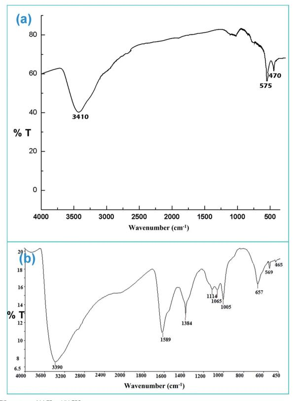
Fig. 1 FTIR spectrum of (a) ZF and (b) ZFC.
