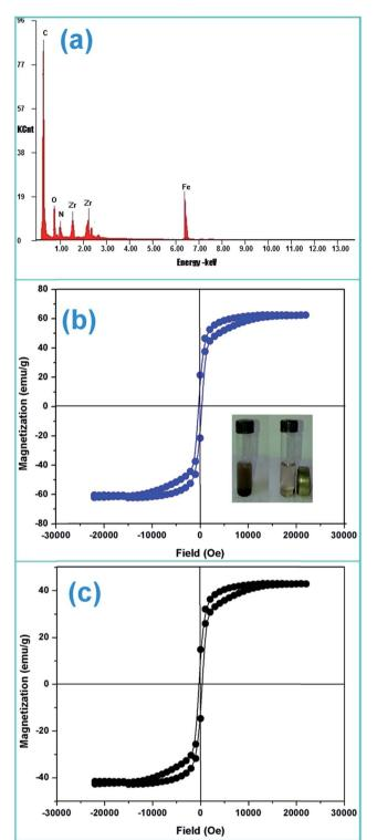
Fig. 4 (a) EDX pattern of ZFC, (b) M-H curve for ZF and (c) M-H curve of ZFC.
