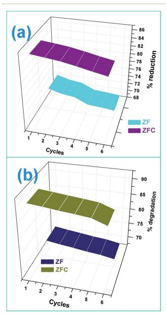
Fig. 10 (a) Reusability of ZF and ZFC for  $Cr(v_i)$  reduction and (b) reusability of ZF and ZFC for 4-CP degradation under solar light.
