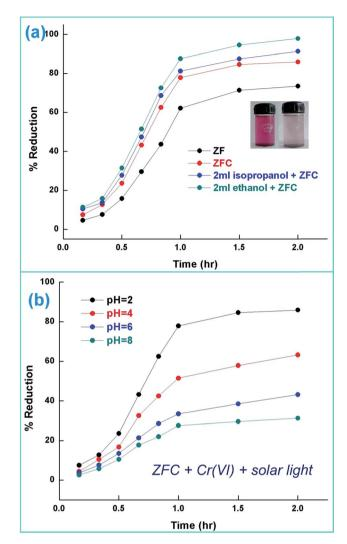
Fig. 7 (a) Photoreduction of Cr(v<sub>1</sub>) under solar light [initial pH 2],  $Cr(v_1) = 70 \text{ mg L}^{-1}$  [temperature = 30  $\pm$  0.5 °C] and (b) ZFC performance as photocatalyst with pH variation under solar light.
