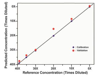
Fig. 5 Calibration and validation data sets of SESORS quantitative measurements of BPE functionalized SERS nanotags through bone.<sup>53</sup> (Reprinted with permission from B. Sharma, K. Ma, M. R. Glucksberg, R. P. Van Duyne, J. Am. Chem. Soc., 2013, 135, 17290 Copyright (2013) American Chemical Society.)
