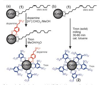
**Scheme 1** Synthesis of water-soluble IONPs by: (a) two-step ligand exchange in solution, leading to exchange of oleic acid ligands  $^{13}$  and (b) herein demonstrated one-step mechanochemical solvent-free process.
