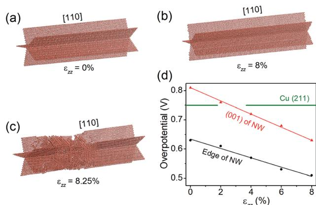
Fig. 6 (a–c) The atomic structure of the penta-twinned Cu NW under  $\varepsilon_{zz} = 0\%$ ,  $8\%$  and  $8.25\%$ . Only the twin boundaries and other lattice defects are shown. (d) Overpotential on the NW edge and (001) facet as functions of uniaxial tension  $\varepsilon_{zz}$ . The green horizontal line indicates the overpotential on the Cu (211) surface.
