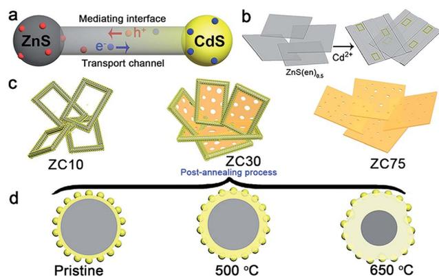
**Scheme 1** (a) Scheme of the mechanism for improving charge-carrier transport in a ZnS/Zn<sub>1-x</sub>Cd<sub>x</sub>S/CdS heterojunction. (b) Schematic illustrating the structural evolution of the mesoporous nanoframe derived from ZnS(en)<sub>0.5</sub> nanosheets. (c) Morphology of ZCX samples with different Cd<sup>2+</sup> content. (d) Effect of the post-annealing process on the microstructure of ZC30.
