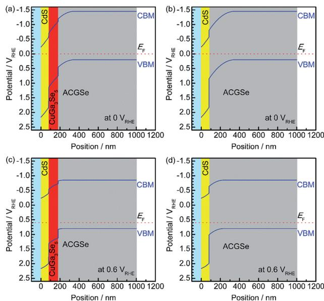
Fig. 8 Calculated band alignment near the solid–liquid interface for CdS/CuGa<sub>3</sub>Se<sub>5</sub>/ACGSe with CuGa<sub>3</sub>Se<sub>5</sub> deposited for 15 min, and Pt/CdS/ACGSe at an applied potential of 0 V<sub>RHE</sub> (a) and (b), and 0.6 V<sub>RHE</sub> (c) and (d). VBM, CBM and E<sub>F</sub> denote the valence-band maximum, conduction-band minimum, and Fermi energy, respectively.
