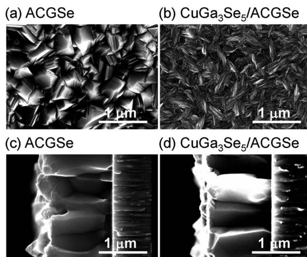
**Fig. 6** Top and cross-sectional SEM images of ACGSe (a) and (c), and CuGa<sub>3</sub>Se<sub>5</sub>/ACGSe with CuGa<sub>3</sub>Se<sub>5</sub> deposited for 15 min (b) and (d).
