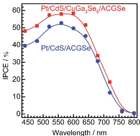
Fig. 2 Wavelength dependence of the IPCE spectra for Pt/CdS/CuGa<sub>3</sub>Se<sub>5</sub>/ACGSe with CuGa<sub>3</sub>Se<sub>5</sub> deposited for 15 min, and Pt/CdS/ACGSe measured at an applied potential of 0 V<sub>RHE</sub>. The IPCE was measured in 0.1 M Na<sub>2</sub>HPO<sub>4</sub> (adjusted to pH 10 by addition of NaOH) under monochromatic light from a 300 W Xe lamp equipped with band-pass filters and an optical fiber.
