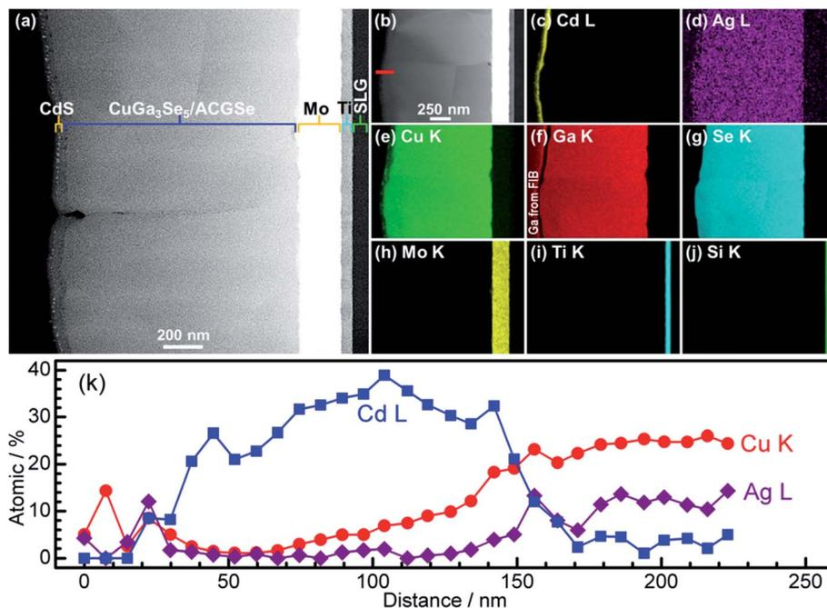
Fig. 7 Cross-sectional TEM images of CdS/CuGa<sub>3</sub>Se<sub>5</sub>/ACGSe sample with CuGa<sub>3</sub>Se<sub>5</sub> deposited for 15 min (a) and (b); EDX elemental maps for Cd (c), Ag (d), Cu (e), Ga (f), Se (g), Mo (h), Ti (i), Si (j); and line profiles for Cd, Cu and Ag across the CdS and CuGa<sub>3</sub>Se<sub>5</sub>/ACGSe interfaces (k). The red line in Fig. 4b indicates where the linear profile was measured. The sample was sliced using a Ga focused ion beam (FIB).
