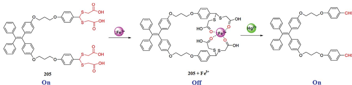
Fig. 171 Chemical structure of ligand 205 and the proposed ligand–metal complexation mechanism.
