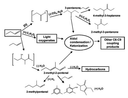
Fig. 7 Proposed reaction mechanism for propanal conversion over Ce<sub>0.5</sub>Z<sub>0.5</sub>O<sub>2</sub> – adapted from Gangadharan et al. 102
