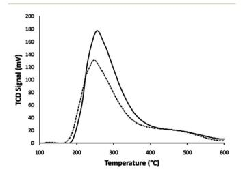
Fig. 9 Ammonia temperature programmed desorption (TPD) for the fresh (solid line) and spent (dotted line) catalyst.<sup>121</sup>
