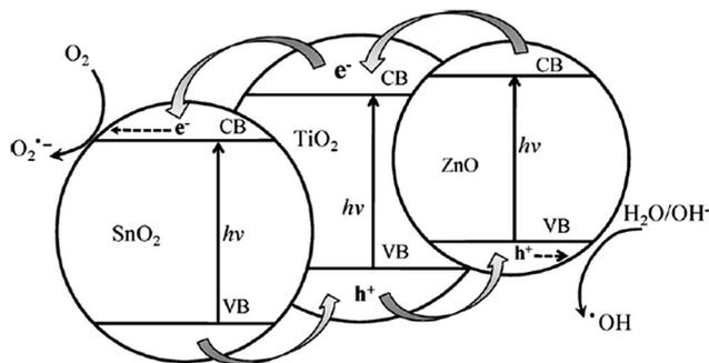
Fig. 14 Energy band structure and electron-hole separation process of a tri-component  $\text{SnO}_2\text{-TiO}_2\text{-ZnO}$  system (reprinted with permission from ref. 227; Copyright 2012 @ Elsevier).
