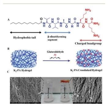
**Fig. 1** Schematic representation of the peptide amphiphile chemical structure (A), peptide gel formation and a glutaraldehyde crosslinking strategy (B), peptide gel (left) and crosslinked peptide gel (right) (C).
