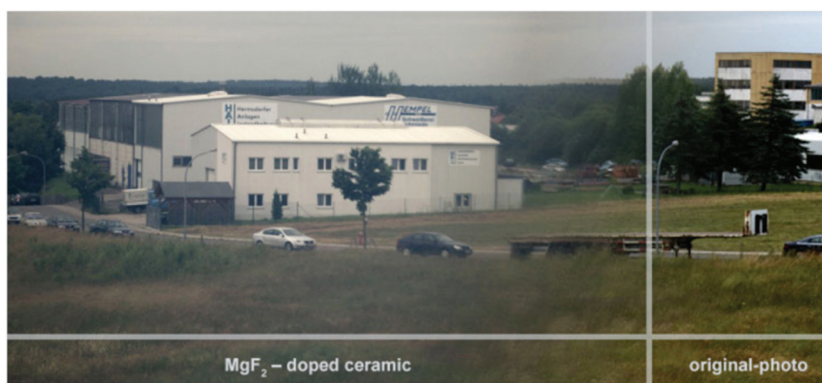
Fig. 17 Picture taken wherein the left side of the camera lens (2/3 of the image) is covered by the “new transparent ceramic” disc whereas the right side shows the original photo.
