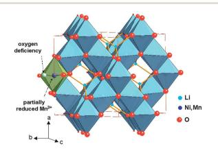
Fig. 1 The structure of spinel  $LiNi_{0.5}Mn_{1.5}O_4$  ( $Fd\bar{3}m$  S.G.). Oxygen deficiency partially reduces  $Mn^{4+}$  to  $Mn^{3+}$  to satisfy local charge neutrality.
