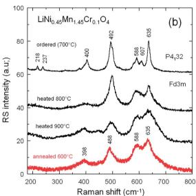
Fig. 5 FTIR (a) and Raman scattering (b) spectra of the LiNi<sub>0.45</sub>Mn<sub>1.45</sub>Cr<sub>0.1</sub>O<sub>4</sub> samples obtained at different steps of the synthesis: at different temperatures up to 900 °C before annealing, and for the final sample, post-annealed at 600 °C for 48 h.
