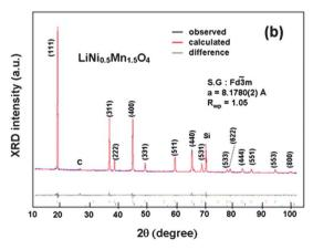
Fig. 3 (a) XRD patterns of the spinel samples at different steps of the synthesis in the temperatures range 700–900 °C before annealing, and for the final sample, post-annealed at 600 °C for 48 h. Inset shows the magnified Bragg lines between  $2\theta=35-45^\circ$  with impurity peaks marked by arrows (b) Rietveld refinement profiles of the XRD data for the LNM electrode film (Si peak comes from sample holder). Reproduced with permission.  $^{64}$
