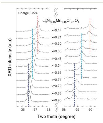
Fig. 13 In situ XRD patterns of the (311) and (511) peaks as a function of x(Li) of Cr-doped LNM spinel during the charge at C/24 rate.
