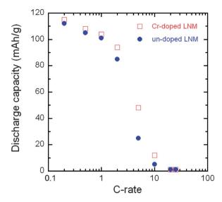
Fig. 12 Modified Peukert curves of LNM and LiNi<sub>0.45</sub>Mn<sub>1.45</sub>Cr<sub>0.1</sub>O<sub>4</sub> spinel cathodes cycled between 3.5 and 4.9 V in CR2032 coin cell with LiPF<sub>6</sub> in EC-DEC (1:1) as electrolyte.
