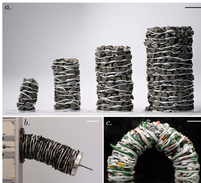
Fig. 1 (a) Elastogranular columns increasing in scale with a fixed volumetric ratio of fibers to grains. Jamming facilitates the formation of elastogranular (a) columns, (b) cantilever beams, and (c) arches. All scale bars 40mm.
