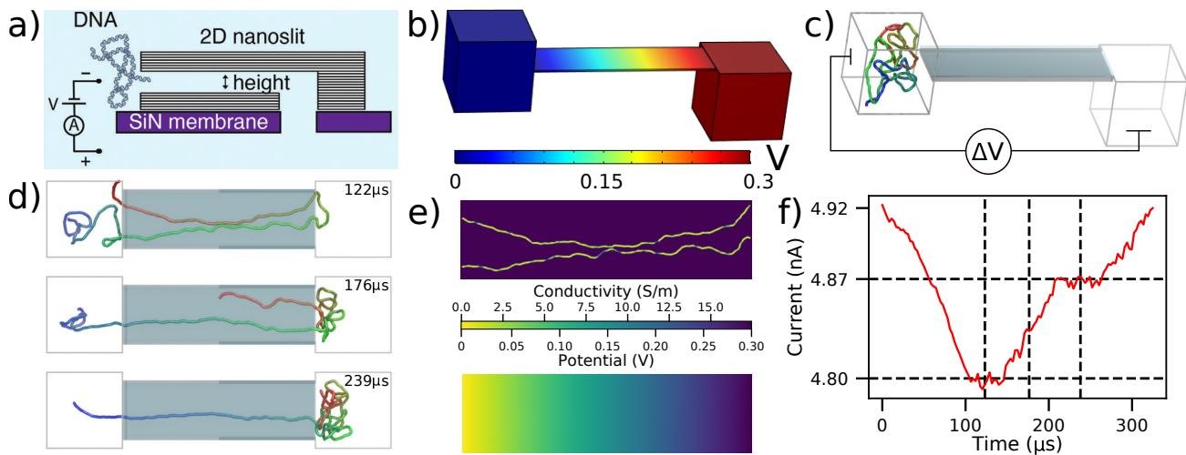
Figure 2: To-scale modeling of the ionic current measured during DNA translocation through a 2D nanoslit.
