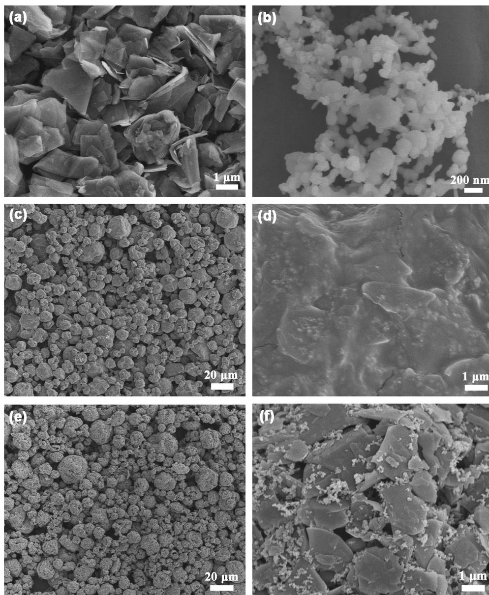
**Fig. 2.** SEM of (a) flake graphite, (b) silicon nanoparticles. (c) spray-dried precursor for Si@FG/C-1 microspheres, (d) enlarged view of (c), (e) Si@FG/C-1, and (f) enlarged view of (e).
