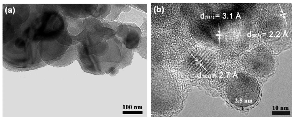
**Fig.3.** (a) TEM and (b) HRTEM images of the Si@FG/C-1.
