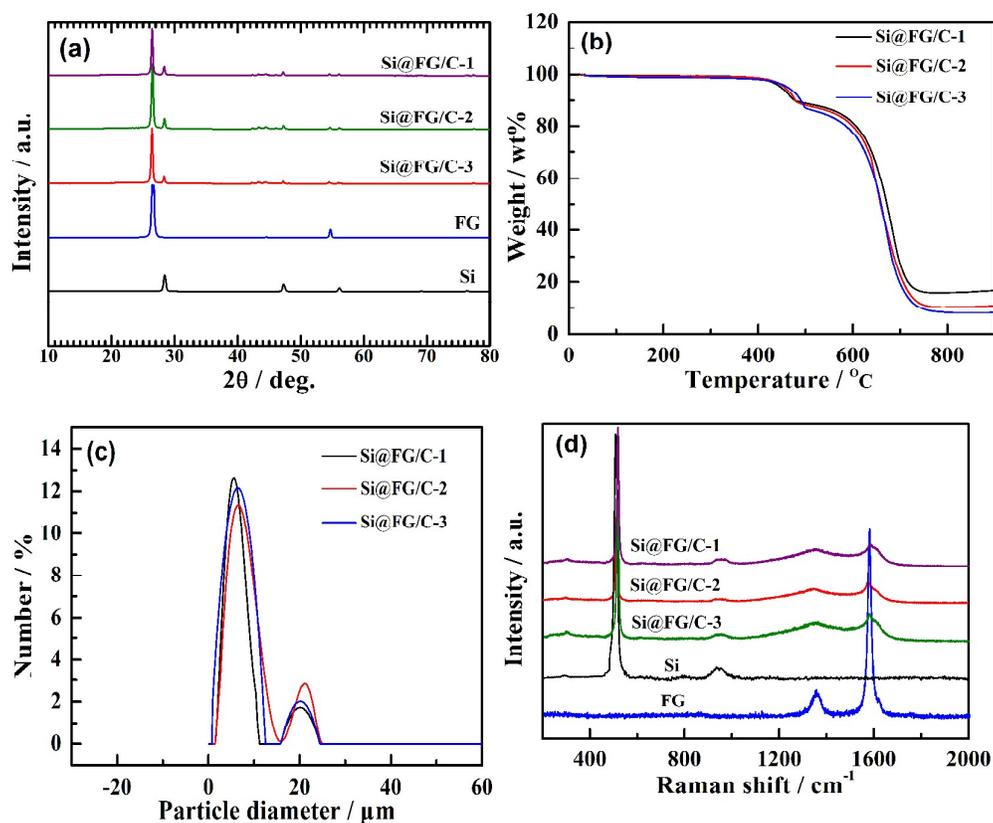
**Fig. 4.** (a) XRD patterns, (b) TG curves, (c) particle size distribution curves, and (d) Raman spectra of the as-received or prepared samples.
