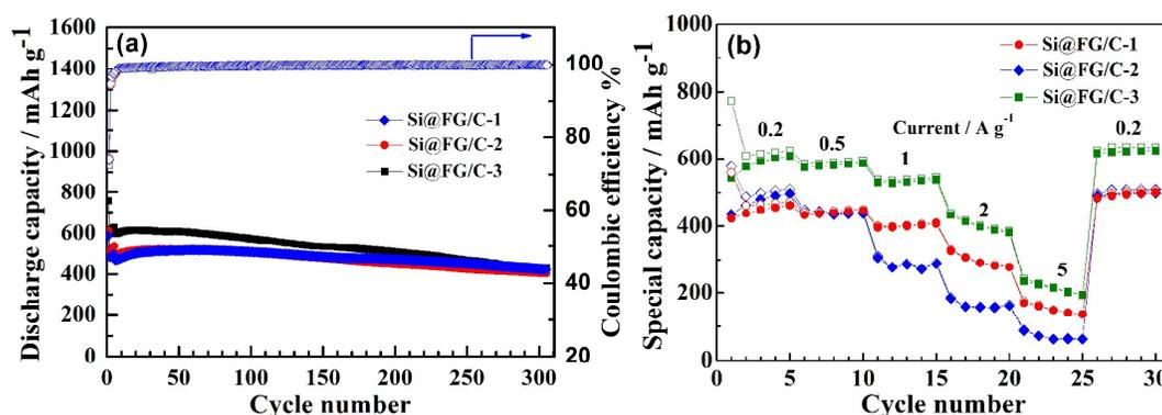
Fig.6. (a) Cycling stability and (b) rate capability of the Si@FG/C composites.
