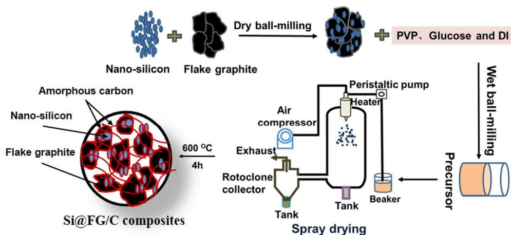
Fig.1. Illustration of the preparation process of Si@FG/C microspheres.
