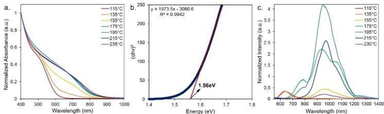
**Figure 4.** a. Absorbance spectra of CuInS<sub>2</sub> NC dispersions in hexanes prepared at different temperatures; b. Tauc plot of the predominantly WZ CuInS<sub>2</sub> NCs prepared at 215°C; c. PL spectra normalized to the QY of CuInS<sub>2</sub> NC dispersions in hexanes prepared at different temperatures.
