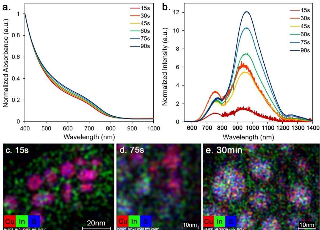
**Figure 7.** a. Absorbance and b. PL spectra of aliquots taken from the synthesis of  $\text{CuInS}_2$  NCs at  $215^\circ\text{C}$ ; c.-d. EDS maps of the 15s and 75s aliquots taken from the synthesis of  $\text{CuInS}_2$  NCs at  $215^\circ\text{C}$ ; e. EDS map of the resultant  $\text{CuInS}_2$  NCs produced by the synthesis for 30 min at  $215^\circ\text{C}$ .
