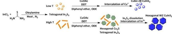
**Figure 1.** Schematic illustration of the synthesis of CuInS<sub>2</sub> NCs.
