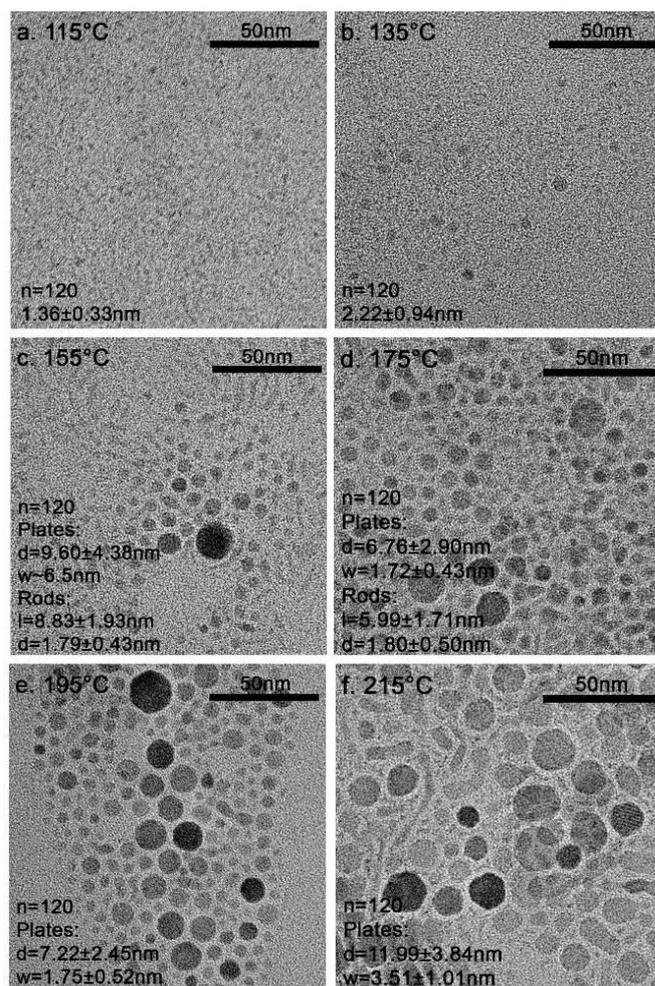
**Figure 2.** a.-f. TEM images of CuInS<sub>2</sub> NCs prepared at reaction temperatures from 115 - 215°C.
