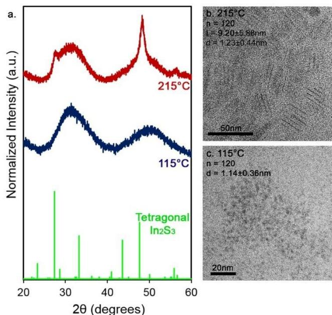
**Figure 5.** a. XRD patterns collected for  $\text{In}_2\text{S}_3$  NCs prepared at 115°C and 215°C. Data for tetragonal  $\beta\text{-In}_2\text{S}_3$  is from JCPDS card no. 25-0390; b.-c. TEM images for precursor  $\text{In}_2\text{S}_3$  NCs prepared at 215°C and 115°C respectively.
