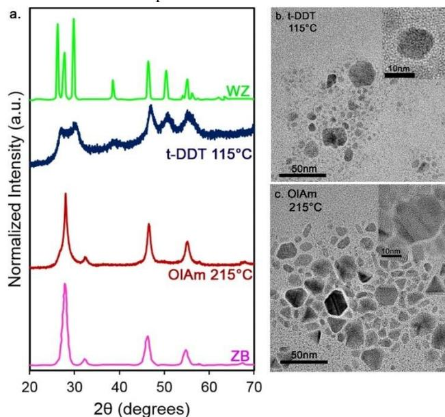
**Figure 6.** a. XRD patterns collected for  $\text{CuInS}_2$  NCs prepared with OIAm as the injection solvent at 215°C and *t*-DDT as the injection solvent at 115°C. Pure ZB and WZ spectra are digitized from the work of Chang *et al.*<sup>36</sup> b.-c. TEM images collected for samples prepared with *t*-DDT injection at 115°C and with OIAm injection at 215°C respectively.
