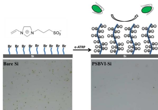
Grafting zwitterionic polymer brushes via electrochemically mediated-surface initiated atom transfer radical polymerization for antibacterial and antifouling applications.
