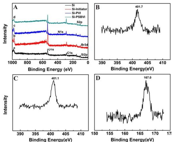
**Fig. 2** (A) XPS survey spectra of bare silicon wafers, initiator-modified silicon wafers, pVI-modified silicon wafers and pSBVI-modified silicon wafers. N 1s XPS spectra of pVI-modified silicon wafers (B) and pSBVI-modified silicon wafers (C). (D) S 2p XPS spectra of pSBVI-modified silicon wafers.
