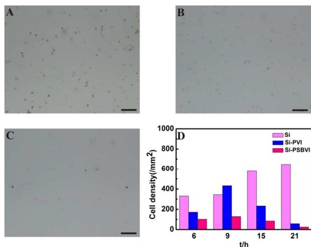
**Fig. 6** Image of *Nannochloropsis maritima* settled on (A) bare Si, (B) Si-pVI and (C) Si-pSBVI after in the *Nannochloropsis maritima* culture suspension for 21 h (scale bars = 50 $\mu$ m). (D) The microalgae settlement data on bare Si surface, pVI and pSBVI brushes coating Si surfaces in different time.
