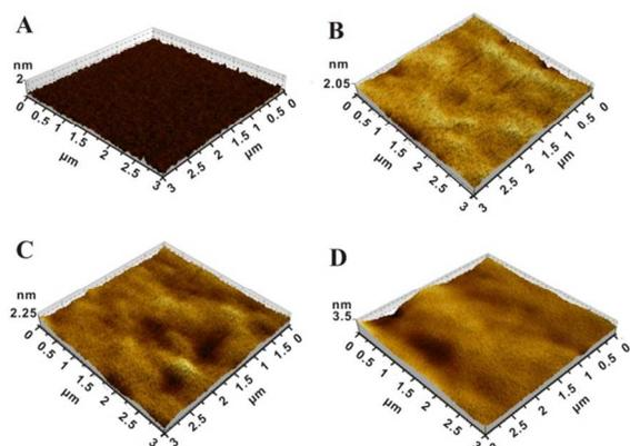
**Fig. 3**  $3 \mu\text{m} \times 3 \mu\text{m}$  AFM 3D images of bare Si before (A) and after modification with (B) initiator, (C) pVI and (D) pSBVI.
