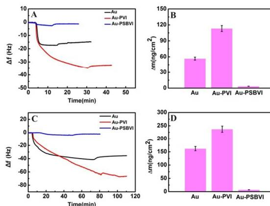
**Fig. 5** The adsorption curves of bare QCM chips, QCM chips modified with pVI and pSBVI brushes in the presence of BSA (A) and lysozyme (C) solutions. The adsorption masses of bare QCM chips, QCM chips modified with pVI and pSBVI brushes in the presence of BSA (B) and Lysozyme (D) solutions.
