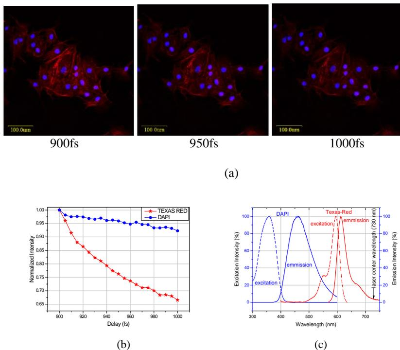
Figure 4: Change in the relative fluorescence intensity of (a) DAPI versus Texas Red, (b) Corresponding fluorescence suppression image of Texas Red relative to DAPI as a function of time delay between pulses under one-color (730 nm) pulse-pair excitation, and (c) Corresponding excitation (broken line) and emission (solid line) spectra of Texas-Red and DAPI relative to the excitation laser wavelength (730 nm) position.
