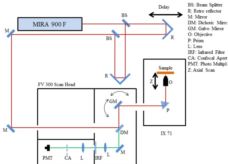
Figure 1: Overall experimental setup used in our experiments. The abbreviations used are expanded in the legend on the side.
