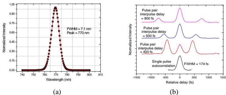
10 Figure 2: (a) Laser pulse spectrum as well as (b) representative autocorrelation trace for pulse pairs at a few different inter-pulse delays are shown. These measurements are made before the pulses enter the microscope.
