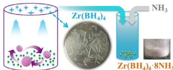
Scheme 1. A schematic illustration of the preparation of  $Zr(BH_4)_4 \cdot 8NH_3$ .
